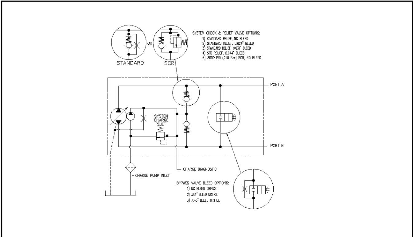
**Figure 3. BDP-10A/21L Standard With Charge Pump Hydraulic Schematic**
