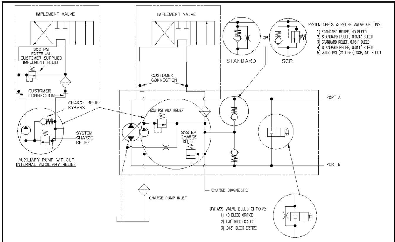
**Figure 4. BDP-10A/21L With Auxiliary Charge Pump Hydraulic Schematic**
