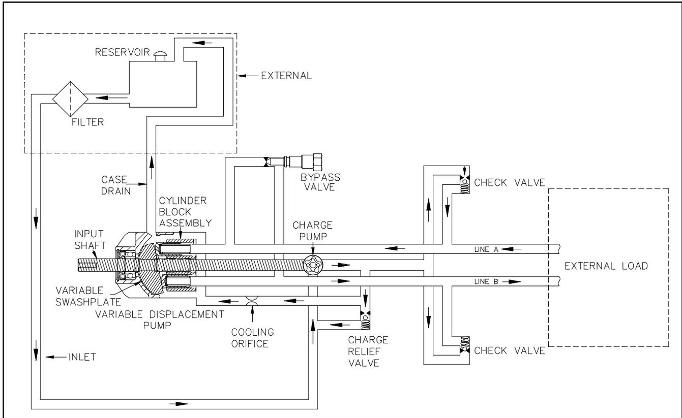
**Figure 5. BDP-10A/21L Standard Charge Pump Graphical Schematic**
