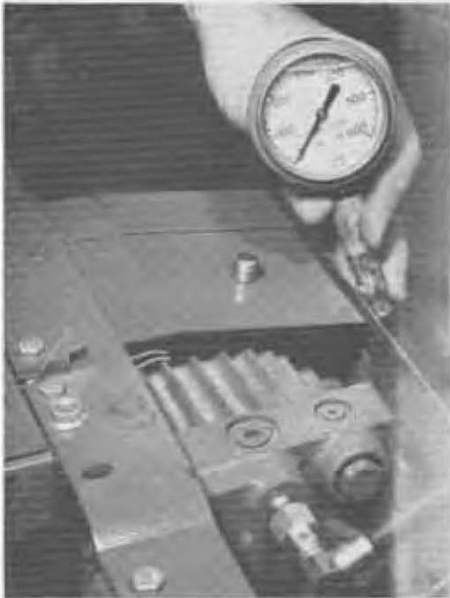
**FIG. 14. Charge Pressure Test — Standard System
