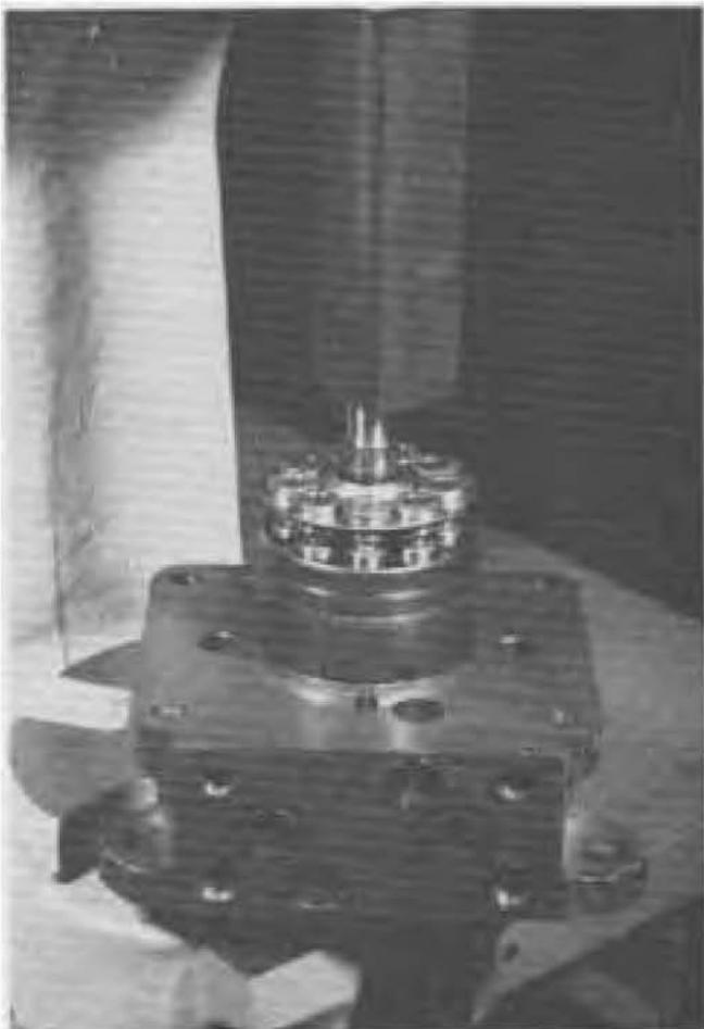
**FIG. 76. Press Motor Shaft to release Retaining Clip**
