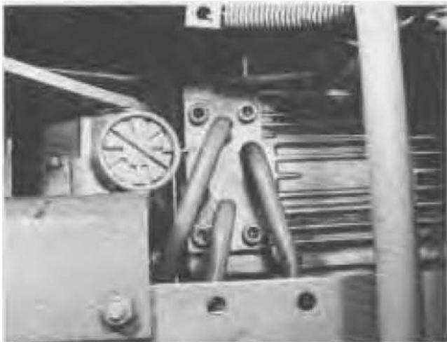
**FIG. 32. Manifold Installed**
