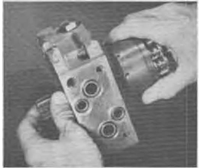
FIG. 85. Install Piston-Cylinder Block Assembly
