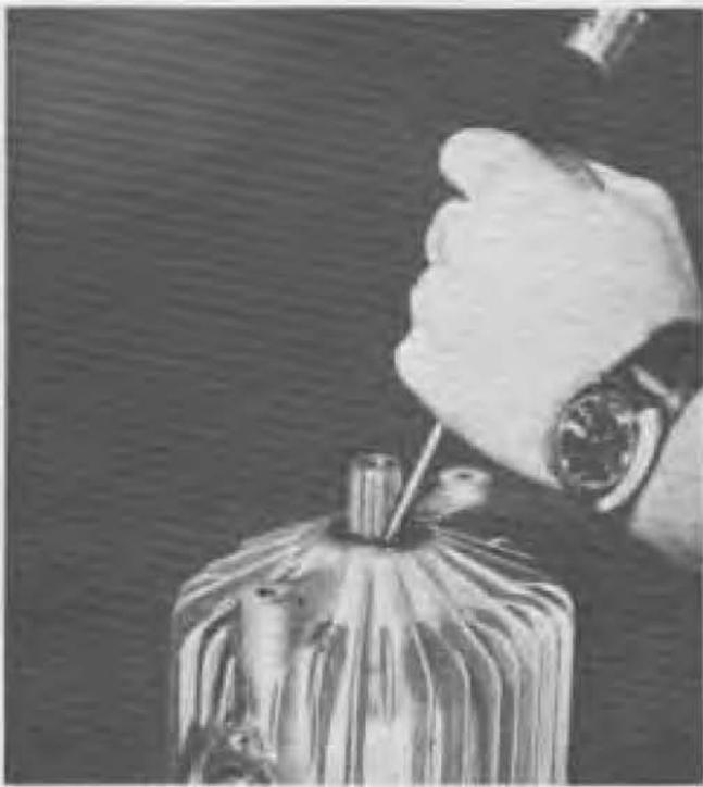
FIG. 55. Seal Removal
