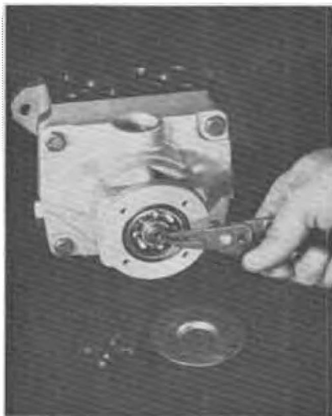
FIG. 71. Remove Snap Ring from Motor Shaft
