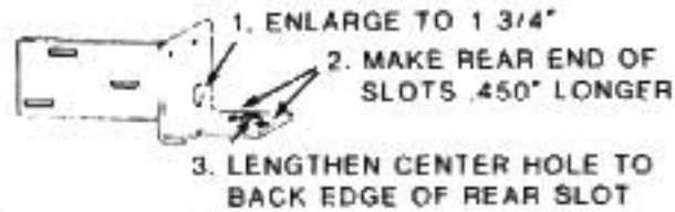
FIG. 3B. Bracket Modification.
