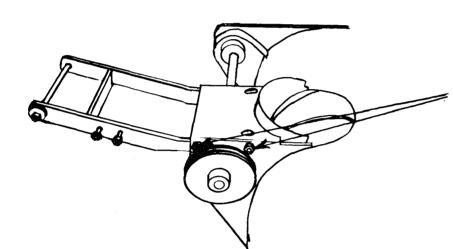
Replace with 3/8-16 x 7/8 bolts or place washers behind bolt to space away from pulley.
