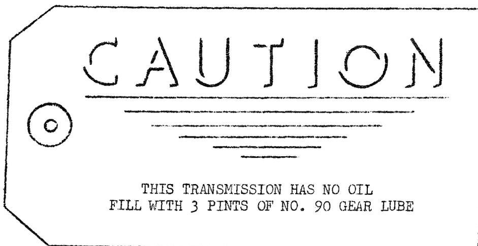
ALL replacement transmissions are also shipped WITHOUT lubricant, IN CARTONS with the shift lever removed for easier packaging. It is suggested that you drain lubricant, remove shift and repack defective unit together with the shift stick in the shipping carton, tagged with a green return tag (furnished by your distributor) and return to your distributor for proper credit.
