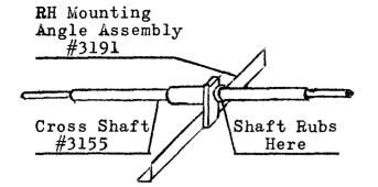
NOTE: The RH Mounting angle assembly, part #3191, in some cases rubs against the cross shaft, #3155, and causes friction.
