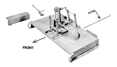
tighten the belt and retighten the stud. 16. To tighten the 30" belt, loosen the nuts on the clutch link. With the mower clutch pedal depressed, turn the rear nut clockwise until belt becomes tight. 17. Lock the other nut against the bracket. CAUTION: Making belts too tight will reduce the life of the belt and bearings.
