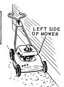
2 Use the left side (the side opposite the chute opening) of your mower when trimming close to buildings, fences, etc.
