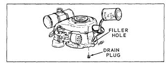
2 Drain and refill the crankcase after the first 5 hours of operating. Thereafter, drain and refill after every 25 hours of operating. Refill crankcase with SAE No. 30 Motor Oil. Fill to top of threads in filler hole. Check oil level of the crankcase before each use, (with mower on level ground). BE SURE DRAIN PLUG IS TIGHT.
