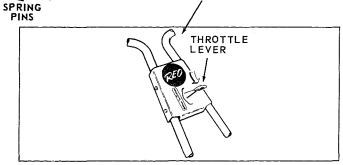
If engine fails to start after repeated attempts, turn the low speed screw and high speed screw clockwise until finger tight. Turn high speed screw counter-clockwise about one full turn and low speed screw counter-clockwise about one and one half turns. Repeat starting operation.
