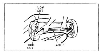
To adjust height of cut, grasp the axle firmly in your hands, using the thumbs against the outside of mower base for leverage, pull axle forward and up or down, releasing into the slots for desired setting. Raising the axles will give a lower height of cut. Lowering the axles will give a higher height of cut.
