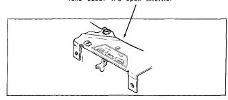
If engine fails to start after repeated attempts, turn the low speed screw and high speed screw clockwise until finger tight. Turn high speed screw counter-clockwise about one full turn and low speed screw counter-clockwise about one and one half turns. Repeat starting operation.
