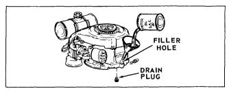
2 Drain and refill the crankcase after the first 5 hours of operating. Thereafter, drain and refill after every 25 hours of operating. Refill crankcase with S.A.E.No. 30 Motor Oil. Fill to top of threads in filler hole. Check oil level of the crankcase before each use, (with mower on level ground). BE SURE DRAIN PLUG IS TIGHT.
