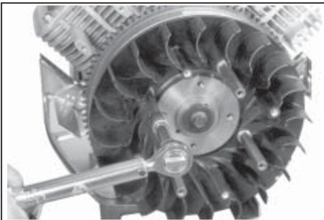
**Figure 11-33. Torquing Supports for Metal Screen (Some Models).**
