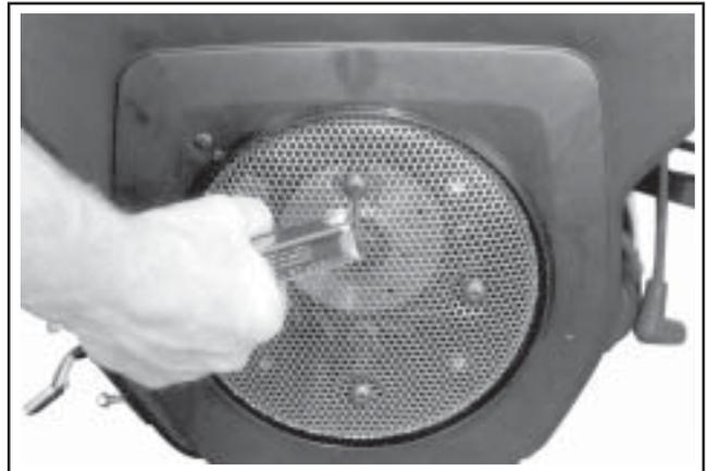
**Figure 9-36. Removing Metal Grass Screen.**
