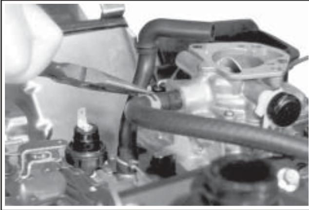
**Figure 9-15. Disconnecting Fuel Inlet Line at Carburetor.**
