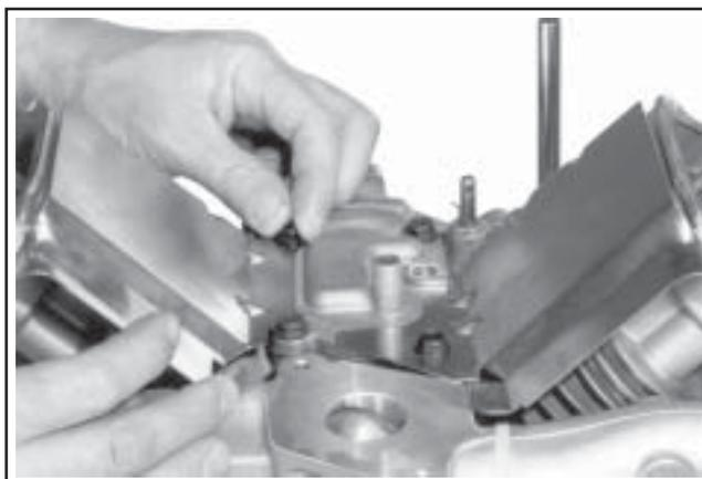
Figure 11-60. Finger Tighten Two Remaining Cover Screws.
