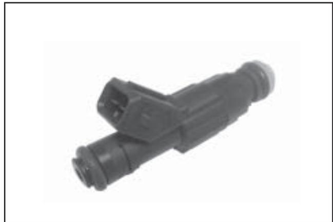
Figure 5B-17. Style 2 Fuel Injector.
