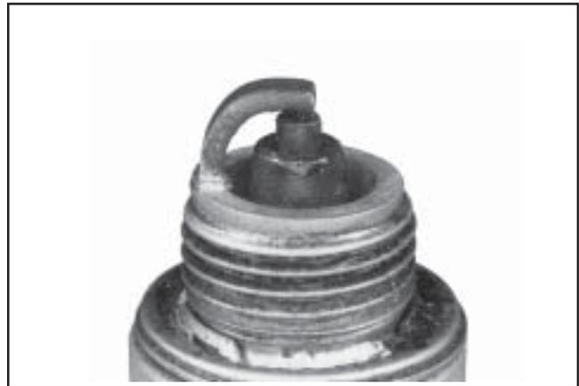
**Wet Fouled:** A wet plug is caused by excess fuel or oil in the combustion chamber. Excess fuel could be caused by a restricted air cleaner, a carburetor problem, or operating the engine with too much choke. Oil in the combustion chamber is usually caused by a restricted air cleaner, a breather problem, worn piston rings or valve guides.
