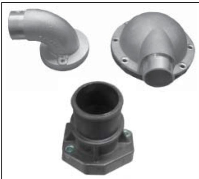
Figure 4-14. Adapters for Heavy-Duty Air Cleaners.
