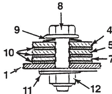
Figure 11-87. Throttle/Choke Control Bracket Detail.
