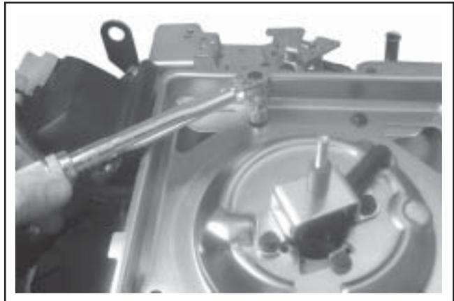
**Figure 11-95. Tightening Rear Base/Bracket Screws (Some Models).**
