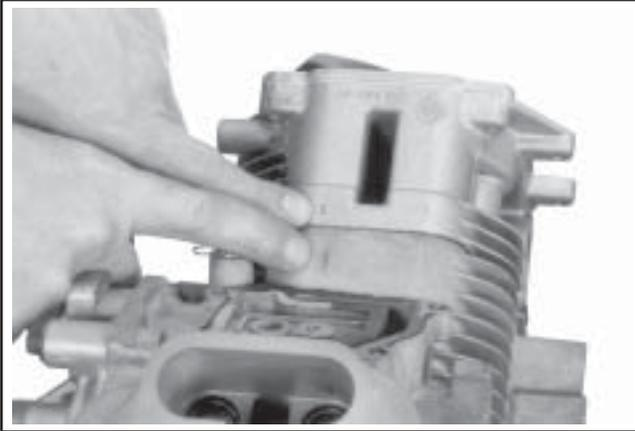
Figure 11-36. Match Numbers on Cylinder Barrel and Head.
