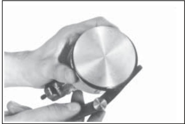
Figure 10-10. Measuring Piston Ring Side Clearance.
