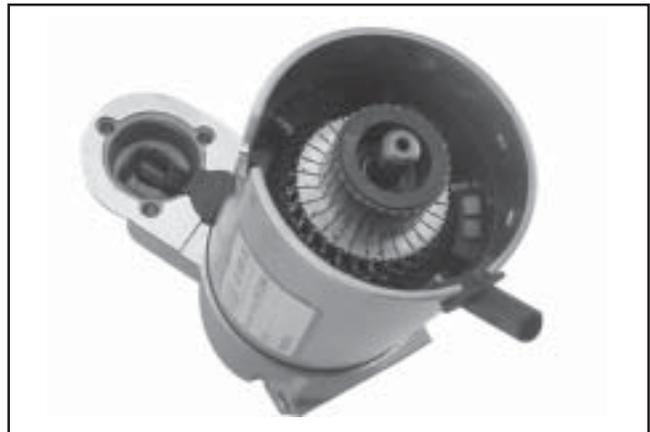
**Figure 8-65. Installing Frame and Drain Tube.**
