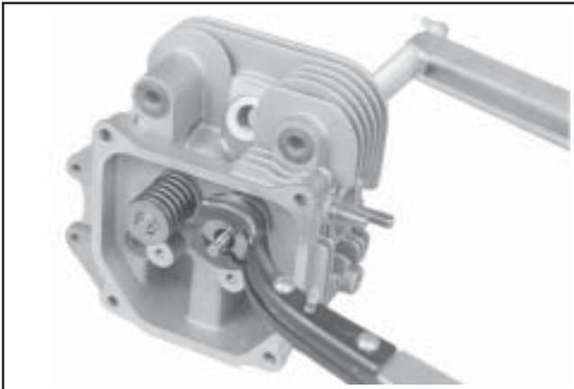
Figure 9-57. Removing Valves with Valve Spring Compressor.
