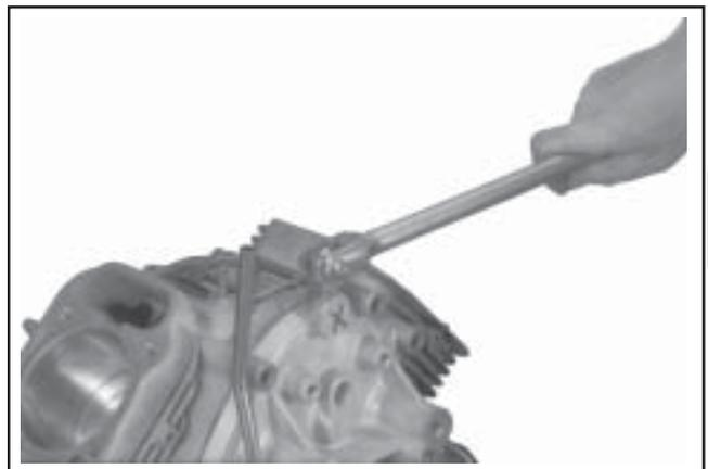
**Figure 9-68. Breaking Seal on Top Splitting Tab.**
