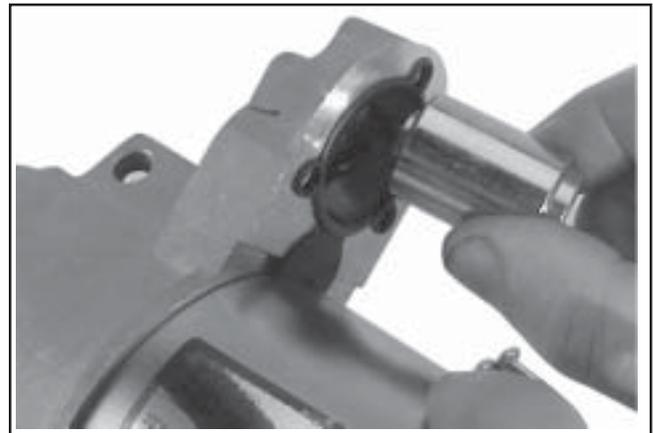
Figure 8-47. Removing Plunger.
