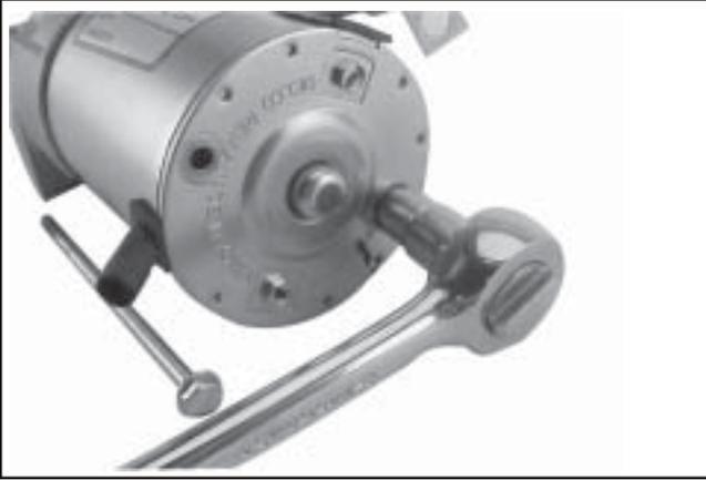
**Figure 8-48. Removing Thru Bolts.**
