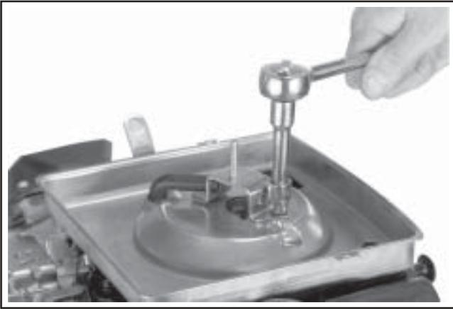
Figure 4-9. Bracket Retaining Screw.
