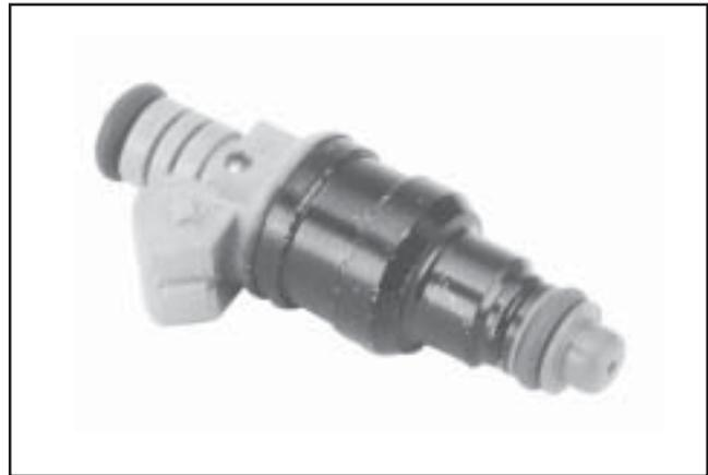
Figure 5B-16. Style 1 Fuel Injector.
