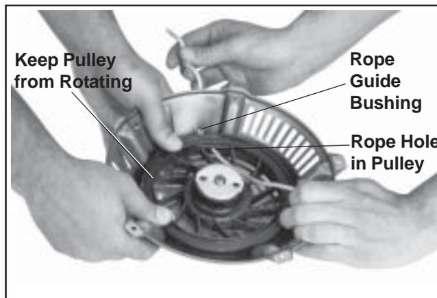
**Figure 7-3. Installing Rope.**
