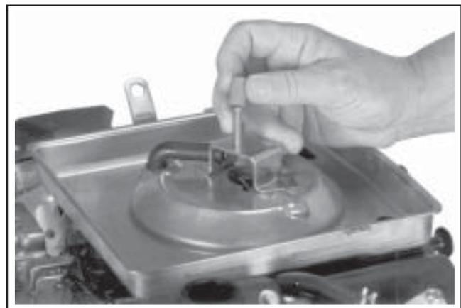
Figure 4-7. Removing Rubber Seal from Bracket.
