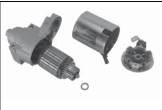
**Figure 8-50. Starter Frame Removed.**
