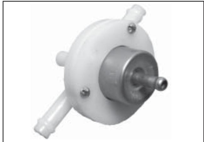
Figure 5B-28. Internal Fuel Pressure Regulator.
