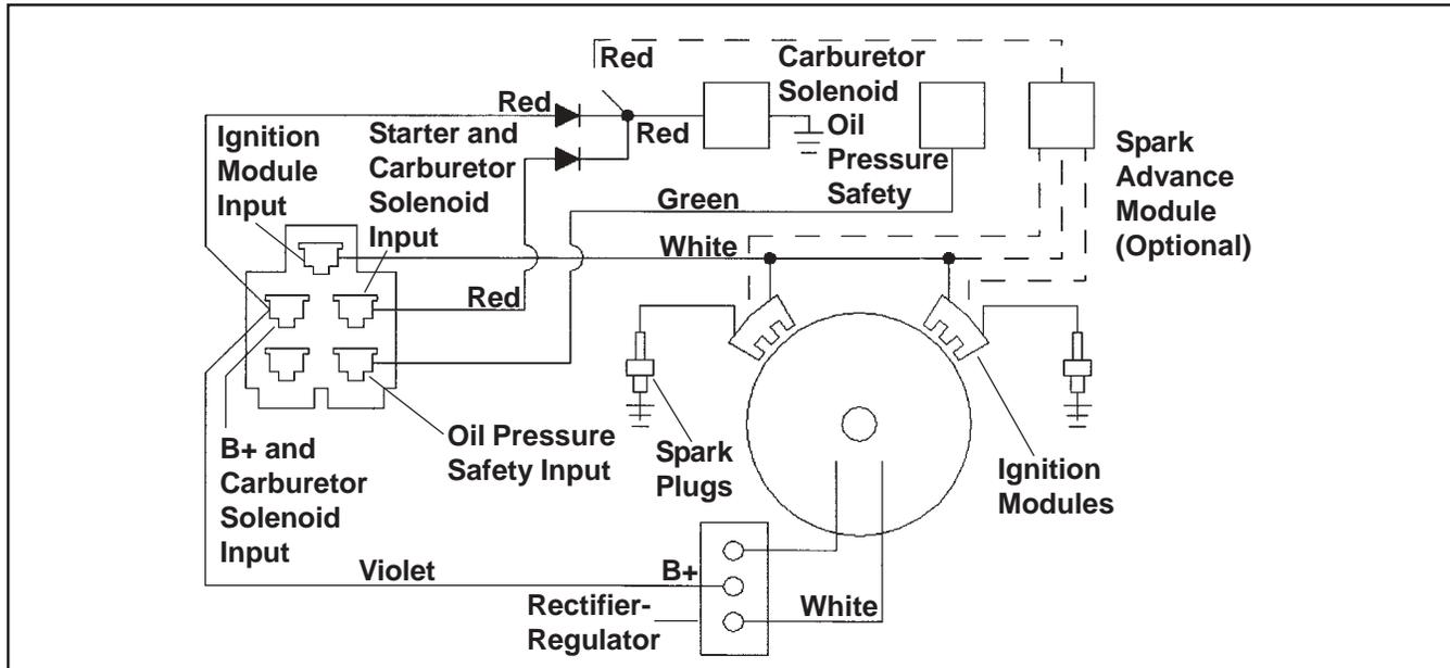
Figure 8-3. Electronic CD Ignition System (For Customer Connected Tractor Applications).
