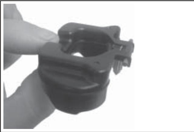
**Figure 5-18. Float and Inlet Needle Details.**
