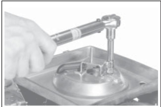
**Figure 11-94. Torquing Base Screws.**
