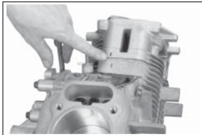
Figure 9-55. Match Marks on Cylinder Barrel and Heads.
