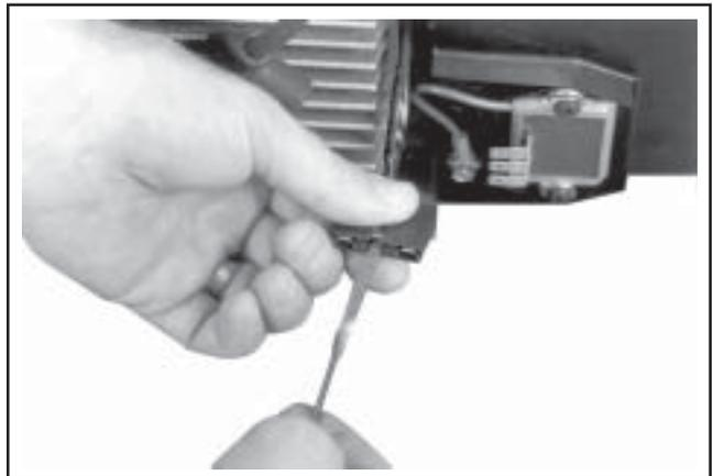
**Figure 9-32. Remove B+ Lead from Terminal Plug.**
