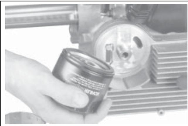
**Figure 11-101. Installing New Oil Filter.**
