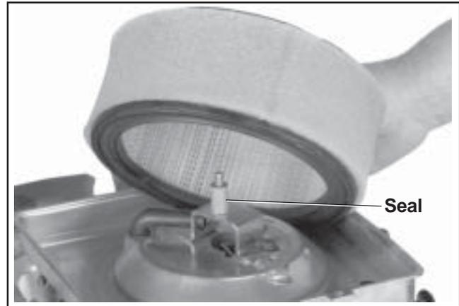
Figure 4-6. Removing Elements.
