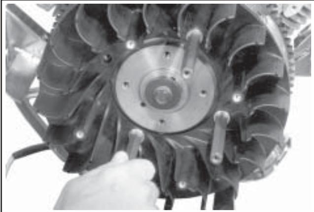
**Figure 11-32. Installing Supports for Metal Grass Screen.**
