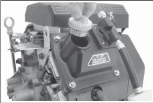
**Figure 6-5. Removing Oil Fill Cap.**
