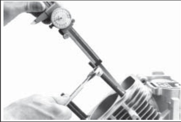
**Figure 11-43. Installing New Mounting Studs to Specified Height.**
