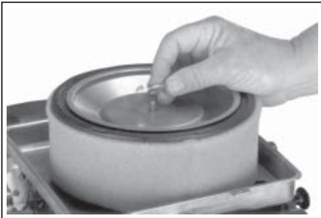
Figure 4-5. Removing Element Cover Wing Nut.
