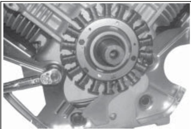
Figure 11-25. Installing Backing Plates and Stator Wire Bracket.
