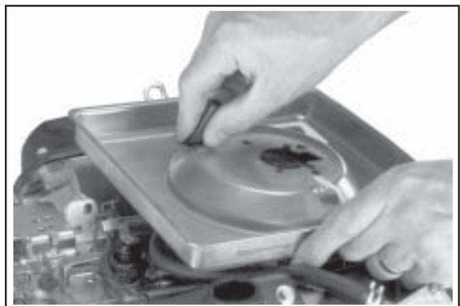
**Figure 9-10. Removing Breather Tube from Base.**
