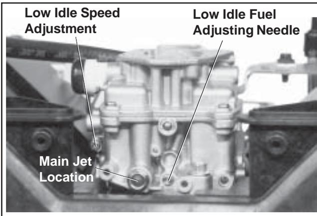
**Figure 5-5. Pre-Compliance Carburetor with Low Idle Adjustment.**
