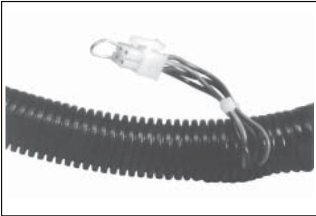
**Figure 5B-8. Service Connector Plug, Metal-Cased ECU Harness.**
