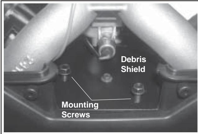
**Figure 9-37. Debris Shield Details (Two-Barrel Carburetor Model Shown).**
