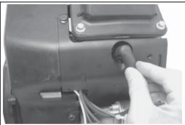
**Figure 11-106. Connect Spark Plug Leads.**
