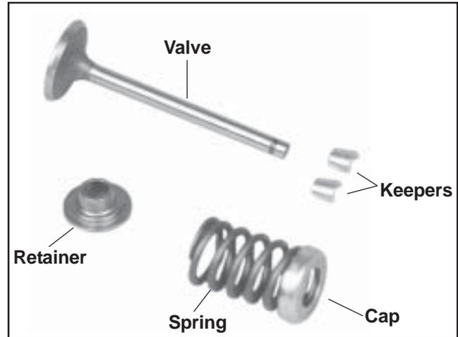
Figure 11-38. Valve Components.
