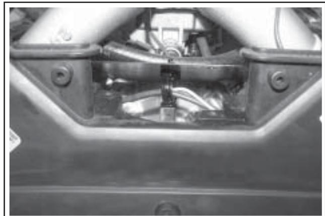
**Figure 11-53. Routing of Wiring Harness (Two-Barrel Models).**
