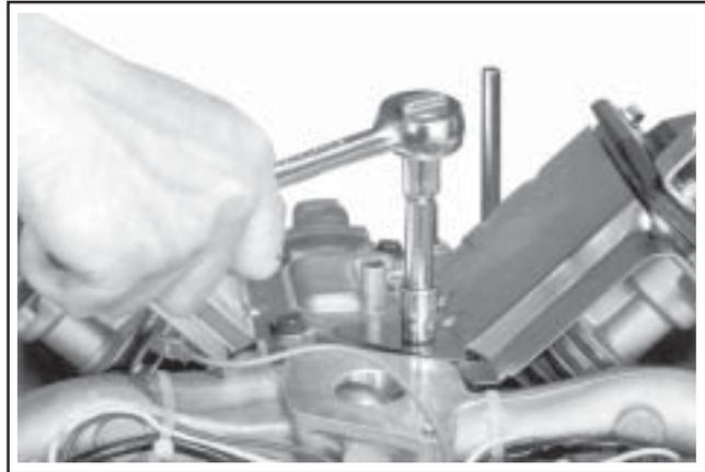
**Figure 9-39. Removing Fasteners Holding Baffle and Breather Cover.**
