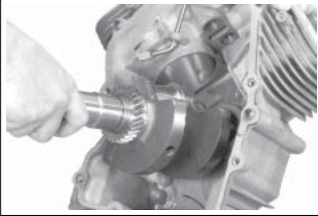
Figure 9-73. Removing Crankshaft.
