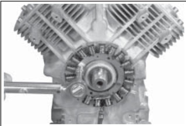
**Figure 9-65. Removing Stator.**
