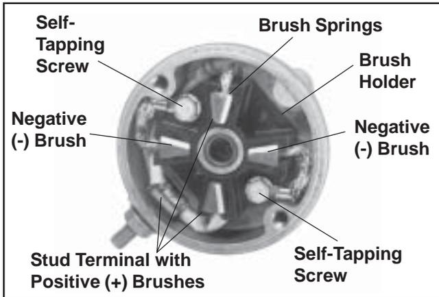
**Figure 8-39. Style "A" Commutator End Cap with Brushes.**
