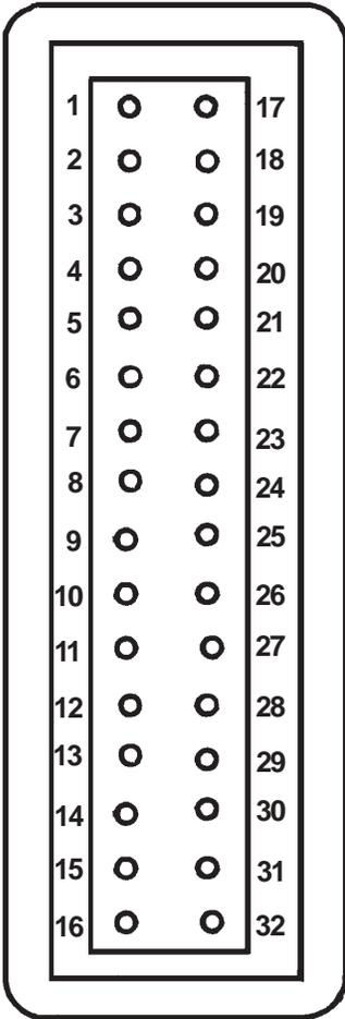
The diagram shows a 32-pin connector with two rows of 16 pins each. The pins are numbered 1 through 32, with the first row containing pins 1-16 and the second row containing pins 17-32. Each pin is represented by a small circle with a dot in the center.
