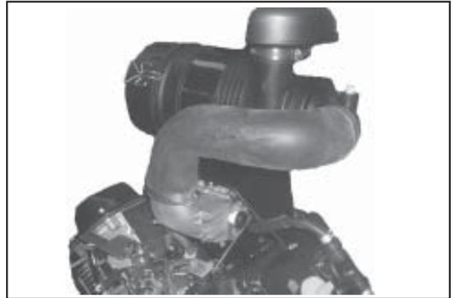
**Figure 11-98. Assembled Heavy Duty Air Cleaner (Two-Barrel Carburetor).**
