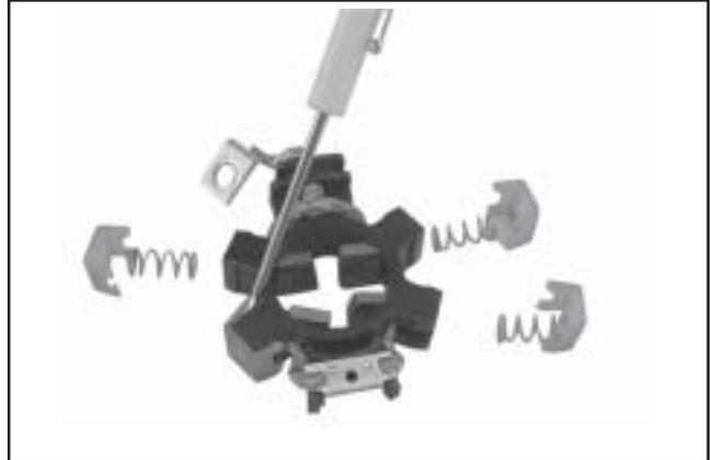
Figure 8-68. Removing Retaining Clips.
