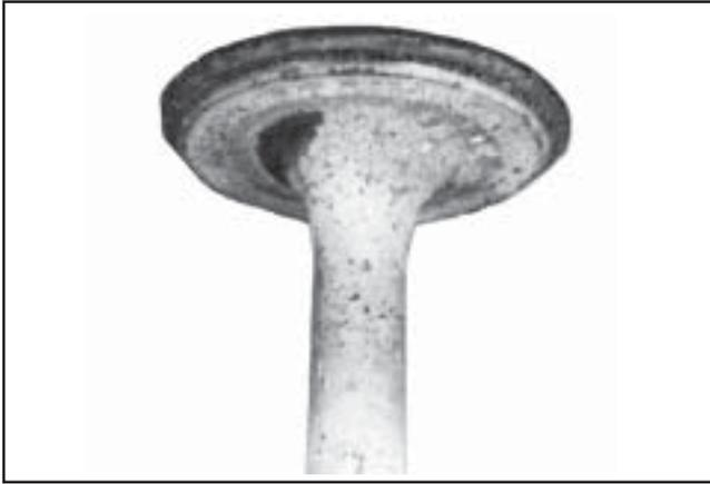
**Normal:** Even after long hours of operation a valve can be reconditioned and reused if the face and margin are in good shape. If a valve is worn to where the margin is less than 1/32" do not reuse it. The valve shown was in operation for almost 1000 hours under controlled test conditions.
