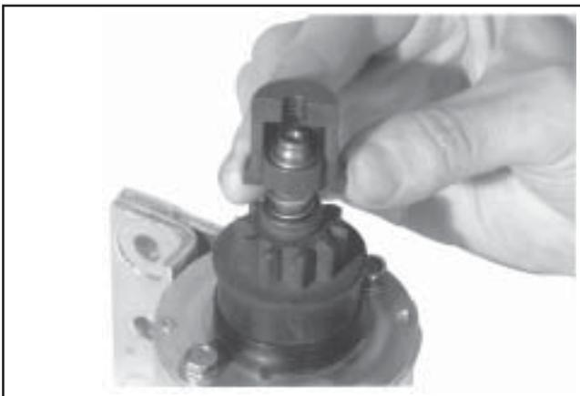
**Figure 8-38. Assembling Larger Inner Half Around Spring Retainer.**
