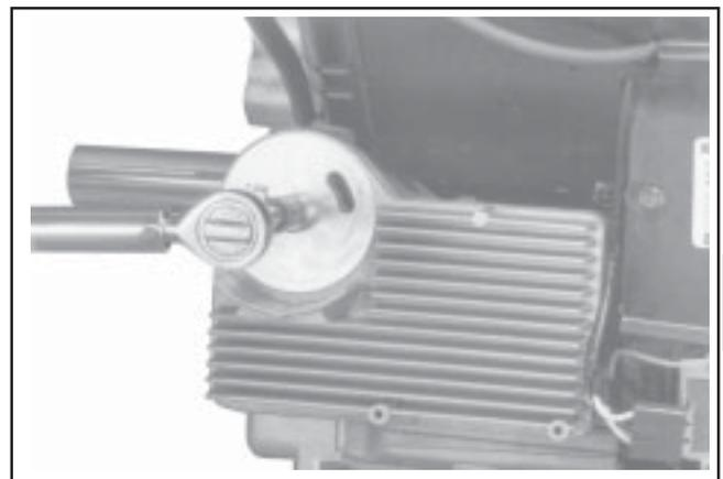
**Figure 11-99. Torquing Oil Filter Nipple (Crankcase Mounted Cooler).**
