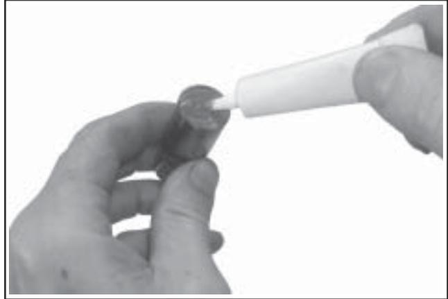
**Figure 11-34. Applying Camshaft Lubricant to Bottom of Lifters.**
