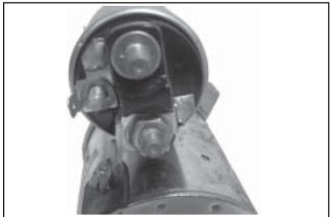
**Figure 8-73. Positive (+) Brush Lead Connection.**
