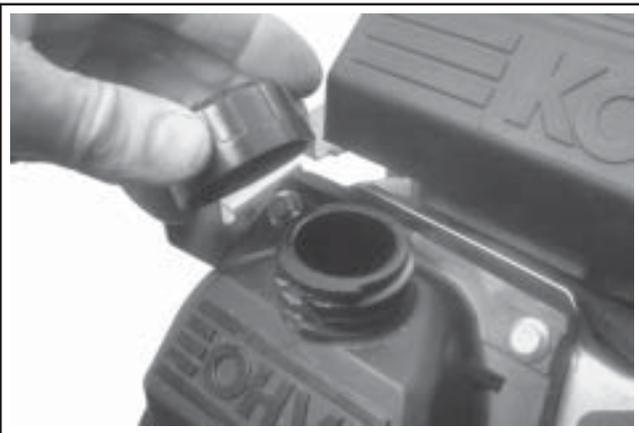
**Figure 11-105. Reinstalling Oil Fill Cap (Some Models).**
