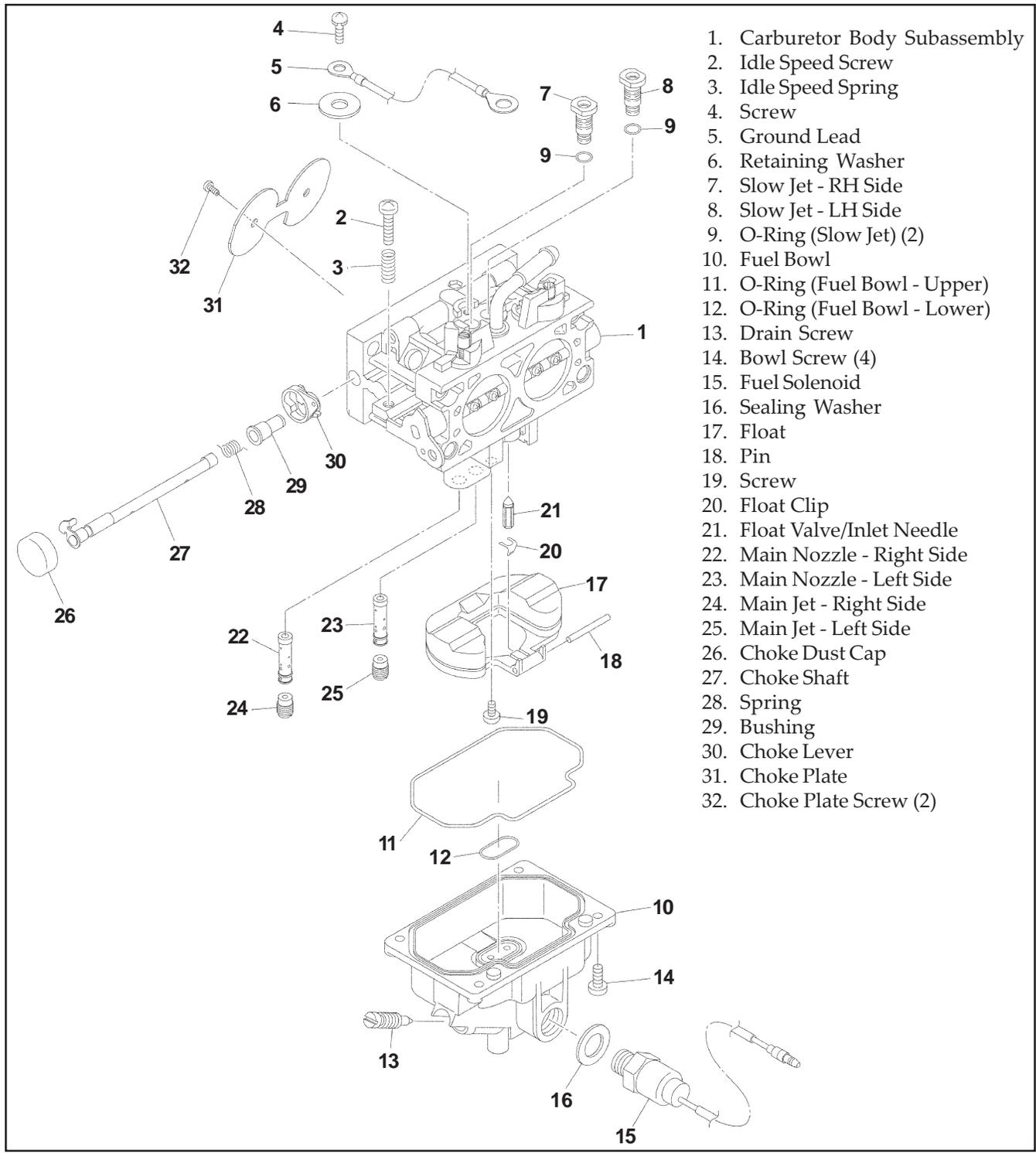
Figure 5-38. Keihin BK Two-Barrel Carburetor - Exploded View.
