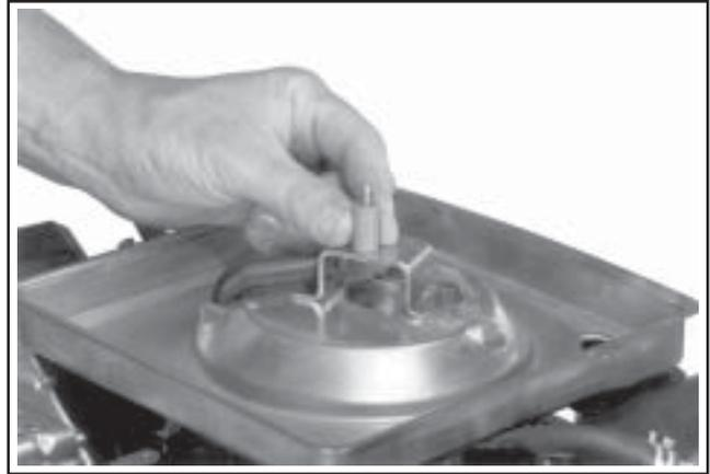
**Figure 9-8. Removing Air Cleaner Base Retainer.**
