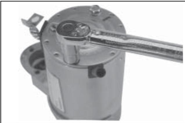
**Figure 8-71. Torquing Thru Bolts.**
