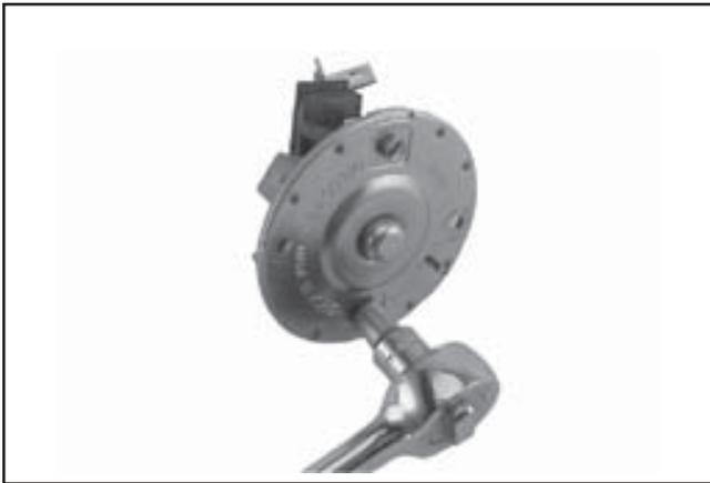
**Figure 8-59. Removing Brush Holder.**
