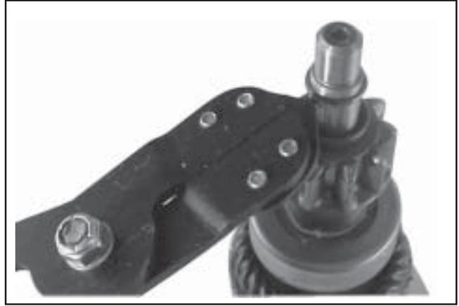
Figure 8-54. Removing Retaining Ring.
