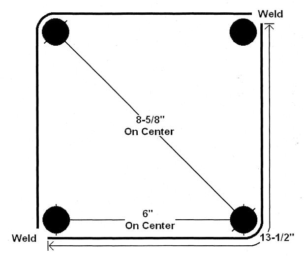
The two steel plates are 3" wide 1/8 of an inch thick. 13-1/2 inches in lenth with curve.
