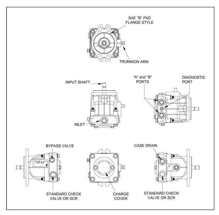
Figure 2. BDP-21L With Standard Charge Pump
