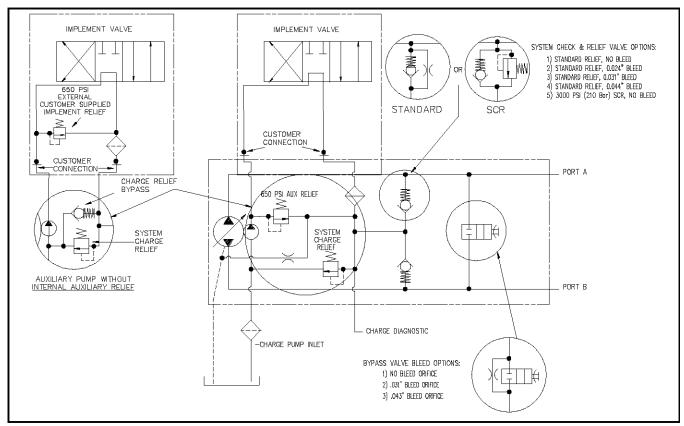
Figure 4. BDP-10A/21L With Auxiliary Charge Pump Hydraulic Schematic
