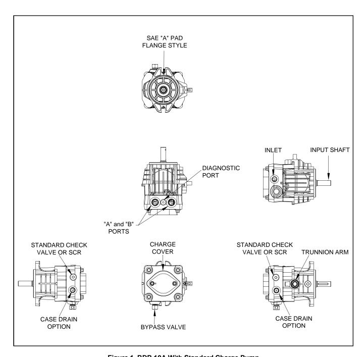
Figure 1. BDP-10A With Standard Charge Pump
