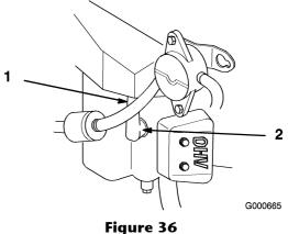
1. Spark plug wire installed 2. Spark plug
