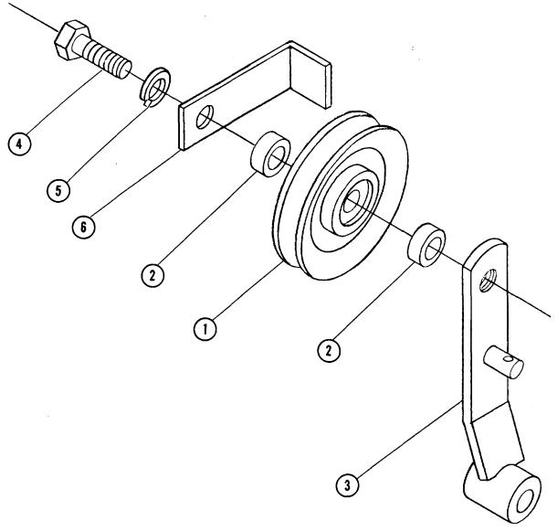
This 6051 idler bracket is for use on 1045 tractor only when mounting a RM-364 mower or SMS-42A sickle bar. The idler bracket which are furnished with these attachments will not work on 1045 tractor.
