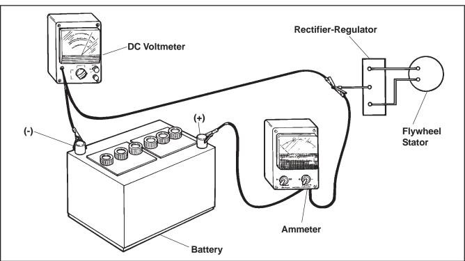
Figure 8-33. Connections for Testing Charging System.
