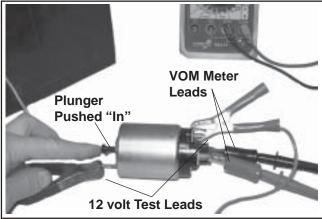
Figure 8-77. Testing Hold-In Coil/Solenoid Contact Continuity.
