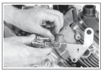
Figure 9-24. Disconnecting Choke Linkage from Actuator Lever.
