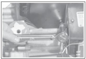
Figure 11-65. Tighten Short Screws to Torque Specified.
