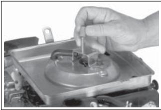
Figure 4-7. Removing Rubber Seal from Bracket.
