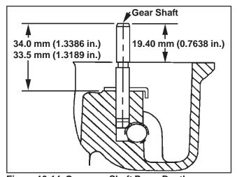
Figure 10-14. Governor Shaft Press Depth.
