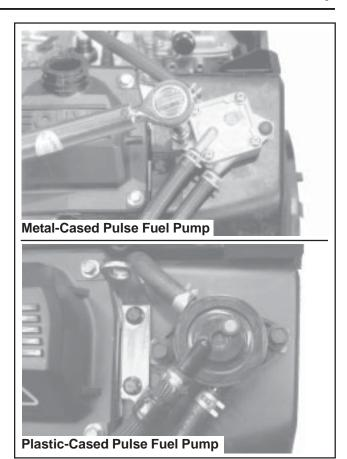
Figure 11-75. Reinstalled Fuel Pump.
