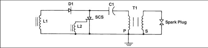
Figure 8-5. Capacitive Discharge Ignition Module Schematic.
