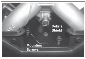
Figure 9-37. Debris Shield Details (Two-Barrel Carburetor Model Shown).
