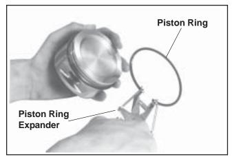
Figure 10-11. Installing Piston Rings.
