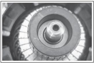
Figure 8-66. Installing Thrust Washer.
