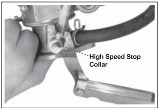
Figure 5A-12. Adjusting/Setting Stop Collar.
