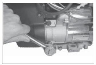
Figure 9-30. Removing Electric Starter Motor.
