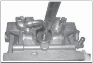
Figure 5-25. Removing Screw and Washer.
