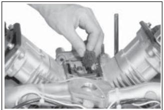
Figure 9-43. Removing Breather Filter.
