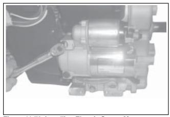
Figure 11-73. Installing Electric Starter Motor.
