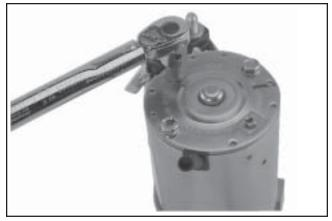
Figure 8-72. Torquing Brush Holder Screws.
