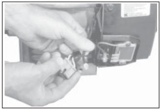
Figure 11-70. Installing B+ Lead into Plug.
