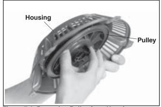
Figure 7-6. Removing Pulley from Housing.
