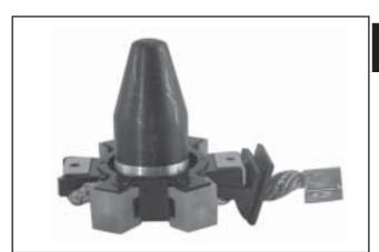
Figure 8-69. Brush Installation Tool with Extension.
