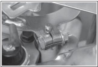
Figure 5B-41. Checking "Split" of Clamp.
