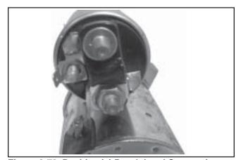
Figure 8-73. Positive (+) Brush Lead Connection.
