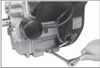
Figure 9-4. Removing Oil Drain Plug.
