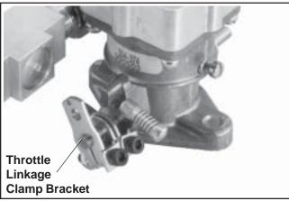
Figure 5A-13. Throttle Linkage Clamp Bracket Position.
