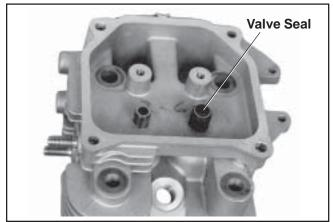
Figure 9-59. Intake Valve Seal Location.
