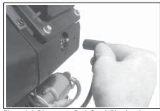
Figure 9-1. Disconnect Both Spark Plug Leads.
