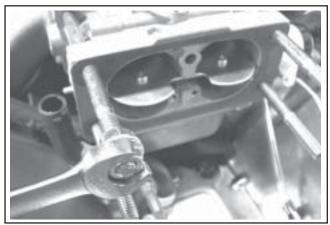
Figure 11-78. Installing Studs and Carburetor (Two-Barrel Carburetor).
