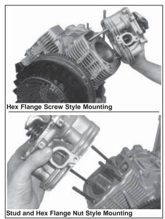
Figure 9-52. Removing Cylinder Head Assembly.
