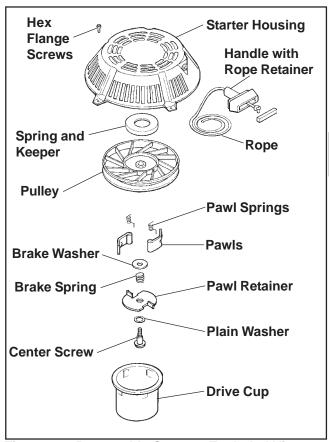
Figure 7-1. Retractable Starter - Exploded View.
