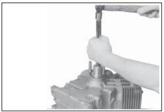
Figure 11-2. Installing Oil Seal.
