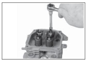
Figure 9-56. Removing Rocker Arms.
