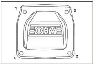
Figure 11-89. Valve Cover Fastener Torque Sequence.
