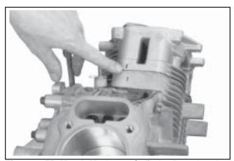
Figure 9-55. Match Marks on Cylinder Barrel and Heads.
