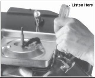
Figure 5B-19. Checking Injectors.
