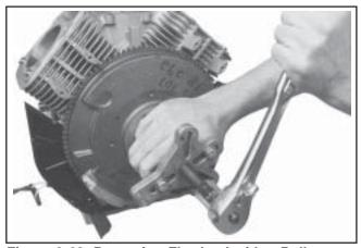
Figure 9-63. Removing Flywheel with a Puller.
