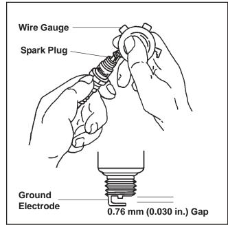
Figure 8-1. Servicing Spark Plug.
