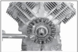
Figure 9-65. Removing Stator.
