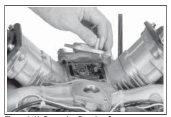
Figure 9-42. Removing Breather Cover.
