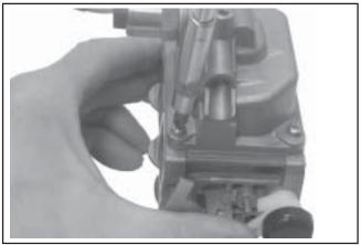
Figure 5-32. Installing Fuel Bowl.
