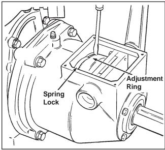
Figure 12-2. Adjusting Clutch.
