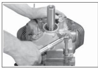
Figure 11-22. Torquing Closure Plate Fasteners.
