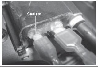
Figure 11-52. Sealant Applied to Terminals.
