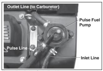
Figure 5-2. Pulse Style Fuel Pump.
