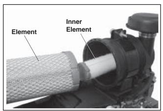
Figure 4-13. Removing Elements.
