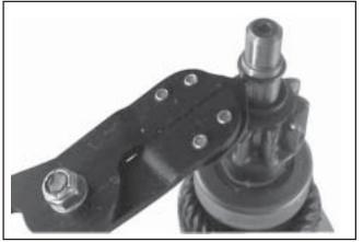
Figure 8-54. Removing Retaining Ring.
