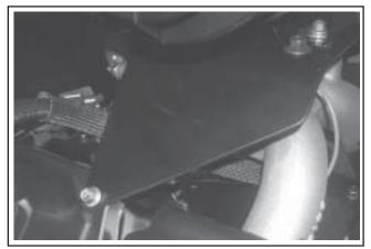
Figure 11-97. Mounted Air Cleaner Bracket (Two-Barrel Carburetor).
