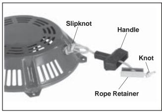
Figure 7-2. Removing Starter Handle.
