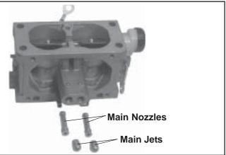
Figure 5-24. Main Jets and Nozzles Removed.
