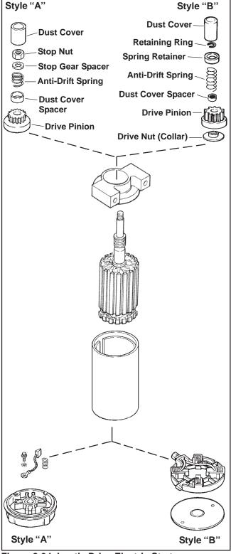
Figure 8-34. Inertia Drive Electric Starter.
