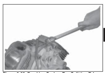
Figure 9-68. Breaking Seal on Top Splitting Tab.
