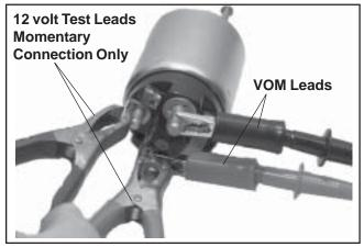
Figure 8-75. Testing Pull-In Coil/Solenoid Contact Continuity.
