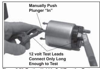
Figure 8-76. Testing Hold-In Coil/Function Test.
