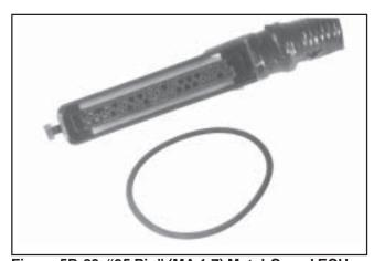
Figure 5B-23. "35 Pin" (MA 1.7) Metal-Cased ECU Connector and O-Ring.
