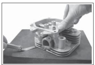
Figure 10-5. Checking Cylinder Head Flatness.
