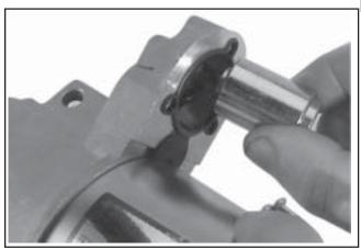
Figure 8-47. Removing Plunger.
