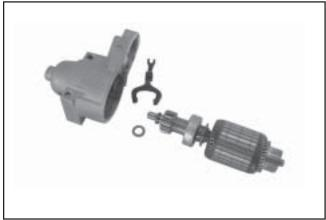
Figure 8-52. Armature and Lever Removed.
