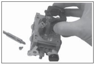
Figure 5-17. Removing Float and Inlet Needle.
