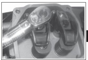
Figure 11-46. Torquing Rocker Arm Screws.
