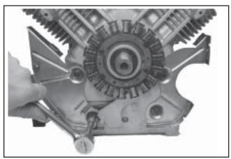
Figure 9-64. Removing Backing Plates and Stator Wire Bracket.
