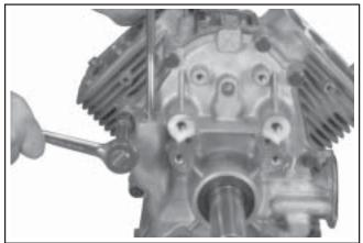
Figure 9-66. Removing the Ten Closure Plate Fasteners.
