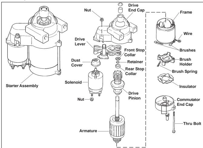
Figure 8-43. Nippondenso Solenoid Shift Starter.
