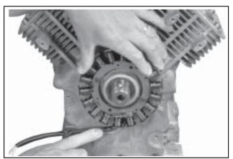
Figure 11-24. Route Stator Leads in Groove.
