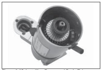
Figure 8-65. Installing Frame and Drain Tube.
