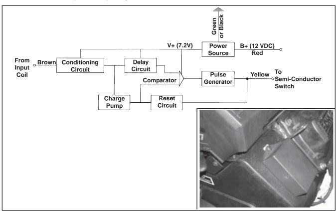
Figure 8-7. Block Diagram - Spark Advance Module.
