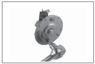
Figure 8-59. Removing Brush Holder.
