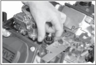
Figure 9-29. Removing Oil Sentry™ Switch from Breather Cover.
