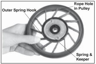
Figure 7-7. Position of Spring and Keeper in Pulley.
