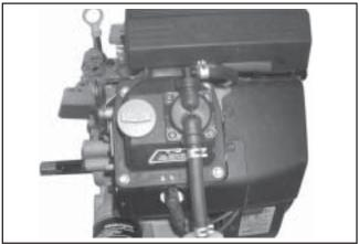
Figure 9-20. Mechanical Fuel Pump.
