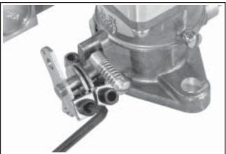
Figure 5A-14. Tightening Throttle Linkage Clamp Bracket.
