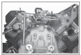
Figure 9-21. Removing Control Bracket.
