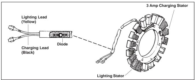
Figure 8-23. 3 Amp/70 Watt Stator.
