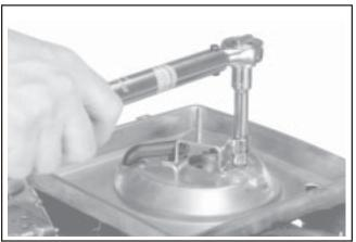
Figure 11-94. Torquing Base Screws.
