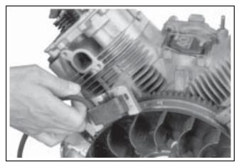
Figure 11-49. Installing Ignition Module.
