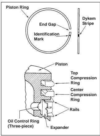
Figure 10-12. Piston Ring Installation.
