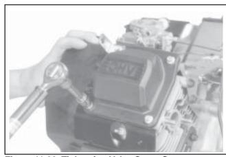
Figure 11-90. Tightening Valve Cover Screws.
