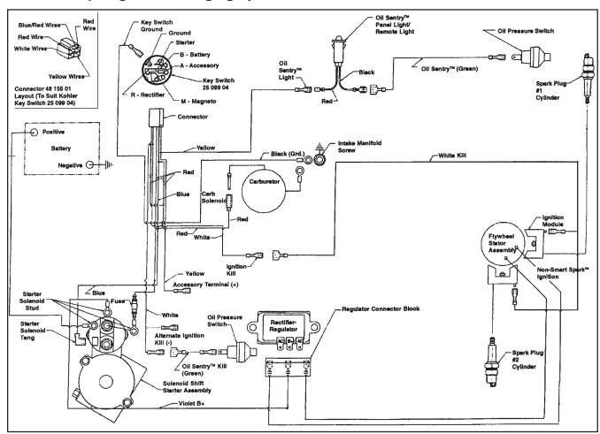
Figure 8-17. Wiring Diagram - 15/20/25 Amp Regulated Battery Charging System with Fixed Timing.
