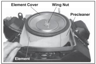
Figure 4-4. Air Cleaner Components.
