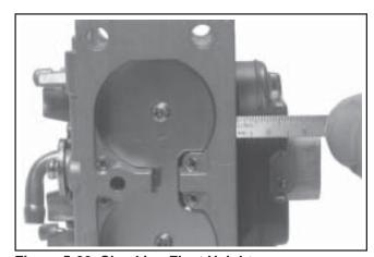
Figure 5-20. Checking Float Height.
