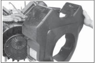
Figure 9-38. Removing Blower Housing.
