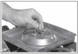
Figure 9-8. Removing Air Cleaner Base Retainer.
