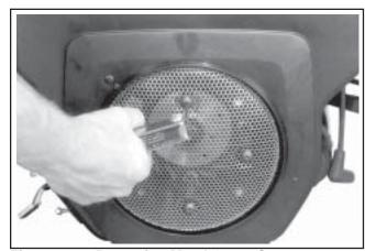
Figure 9-36. Removing Metal Grass Screen.
