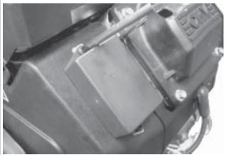
Figure 9-33. Removing the Spark Advance Module (Applicable Models).
