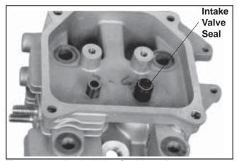
Figure 11-37. Intake Valve Seal Location.
