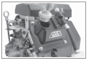
Figure 6-5. Removing Oil Fill Cap.
