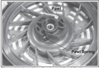
Figure 7-9. Installing Pawls and Pawl Springs.
