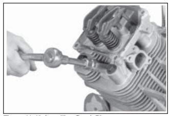
Figure 11-48. Installing Spark Plugs.
