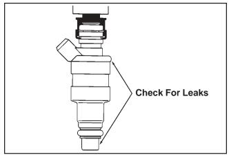
Figure 5B-21. Injector Inspection Points.
