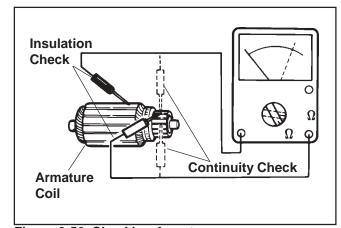
Figure 8-58. Checking Armature.
