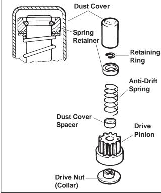
Figure 8-35. Drive Components, "Bonded" Inertia Drive Starter.
