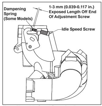
Figure 5B-36. Idle Speed Screw Details.
