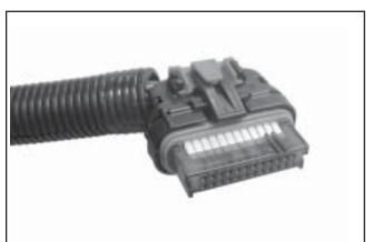
Figure 5B-24. "24 Pin" (MSE 1.0) Plastic-Cased ECU Connector.
