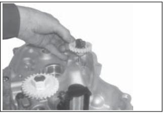
Figure 10-13. Removing Governor Gear.
