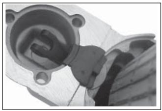
Figure 8-64. Installing Backup Washer and Grommet.
