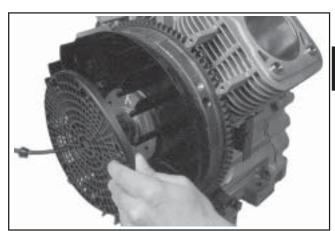
Figure 11-31. Installing Plastic Grass Screen.
