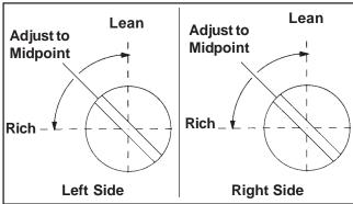
Figure 5-13. Optimum Low Idle Fuel Settings.
