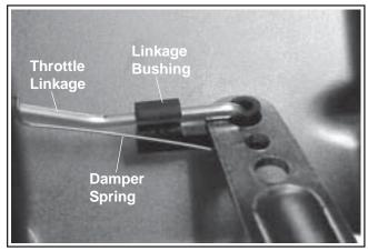
Figure 5B-37. Throttle Linkage/Governor Lever Connection.
