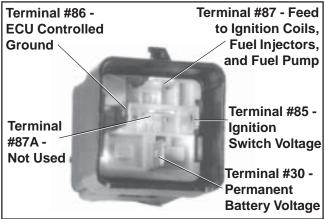
Figure 5B-15. Relay Terminal Details.
