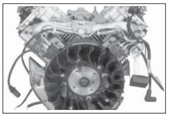
Figure 11-55. Connect Leads on SMART-SPARK $_{\scriptscriptstyle TM}$  Ignition Modules.
