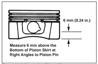
Figure 10-4. Measuring Piston Diameter.
