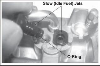
Figure 5-26. Slow Jets and O-Ring Detail.
