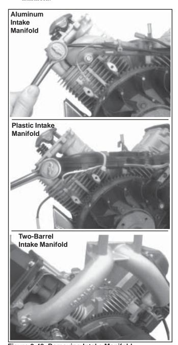
Figure 9-48. Removing Intake Manifold.
