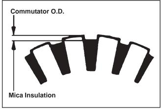
Figure 8-57. Commutator Mica Inspection.
