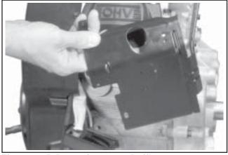
Figure 9-35. Removing Outer Baffles.
