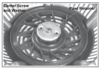
Figure 7-4. Center Screw, Washer and Pawl Retainer.
