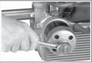
Figure 9-5. Removing Oil Filter.
