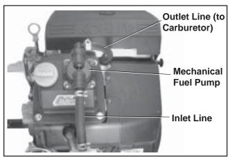
Figure 5-3. Mechanical Fuel Pump.
