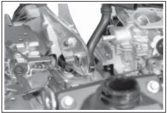
Figure 9-11. Removing Tube from Breather Cover.
