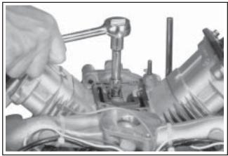
Figure 11-56. Installing Breather Reed Assembly.
