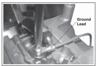
Figure 9-26. Remove Ground Lead (Two-Barrel Model Pictured).
