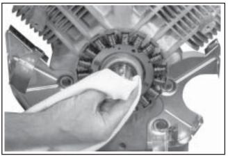
Figure 11-26. Clean and Dry Taper of Crankshaft.
