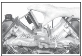
Figure 11-59. Installing Inner Baffles.
