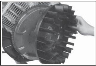
Figure 11-30. Installing Fan on Flywheel.
