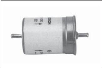
Figure 5B-32. In-Line Fuel Filter.
