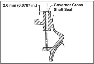
Figure 10-18. Installing Cross Shaft Oil Seal.
