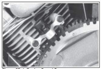
Figure 5B-4. Engine Speed Sensor.
