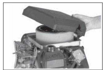
Figure 4-2. Removing Latch Style Cover.
