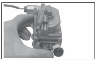
Figure 5-21. Installing Fuel Bowl.
