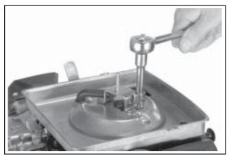
Figure 4-9. Bracket Retaining Screw.
