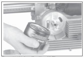
Figure 11-101. Installing New Oil Filter.
