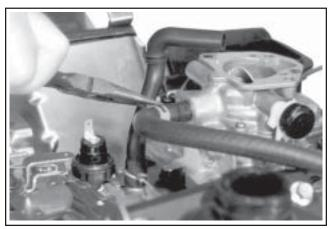
Figure 9-15. Disconnecting Fuel Inlet Line at Carburetor.
