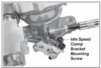
Figure 5A-8. Backing Off Idle Speed Screw.
