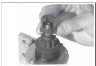
Figure 8-38. Assembling Larger Inner Half Around Spring Retainer.
