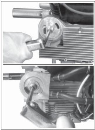
Figure 9-6. Removing Oil Filter Adapter Nipple.
