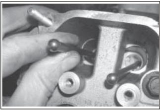
Figure 11-45. Install Push Rods in Their Original Position.
