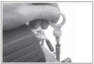
Figure 11-104. Reinstall the Dipstick in Tube.
