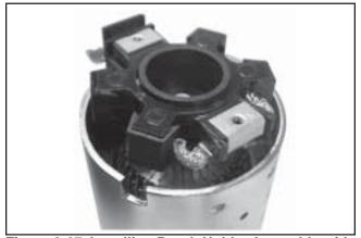
Figure 8-67. Installing Brush Holder Assembly with Supplied Tube.
