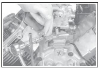
Figure 11-82. Holding and Tightening Governor Arm.
