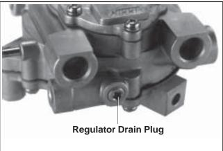
Figure 5A-23. Regulator Drain Plug (Some Models).
