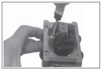
Figure 5-19. Installing Float Assembly.
