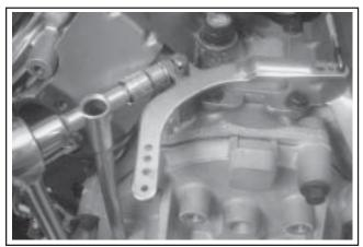
Figure 9-25. Removing Governor Lever.
