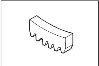
Figure 2-1. Flywheel Holding Tool.
