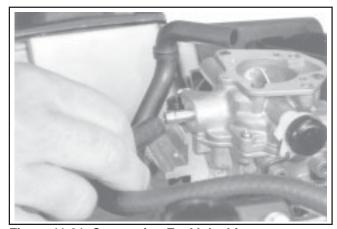
Figure 11-91. Connecting Fuel Inlet Line.
