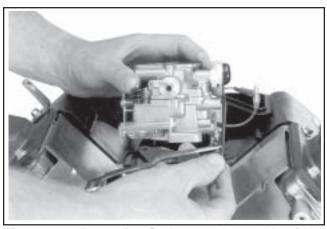
Figure 9-28. Removing Carburetor Assembly with Governor Lever Attached.
