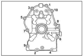
Figure 11-21. Closure Plate Fastener Torque Sequence.
