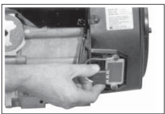
Figure 9-31. Disconnecting Plug from Rectifier-Regulator.
