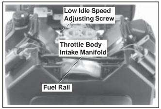
Figure 5B-35. Upper Intake Manifold.
