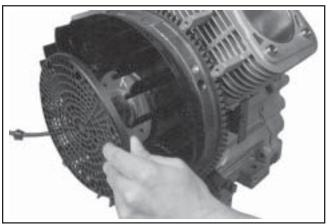
Figure 9-60. Removing Plastic Type Grass Screen.
