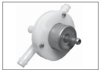
Figure 5B-28. Internal Fuel Pressure Regulator.
