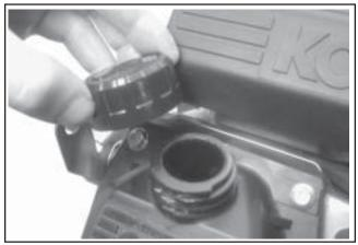
Figure 9-3. Removing Oil Fill Cap from Cover.
