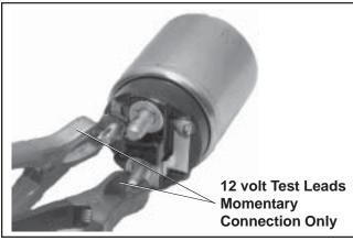
Figure 8-74. Testing Pull-In Coil/Plunger Actuation.
