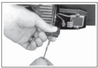
Figure 9-32. Remove B+ Lead from Terminal Plug.
