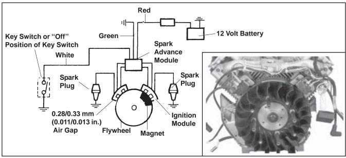
Figure 8-6. Capacitive Discharge Ignition System with Spark Advance.
