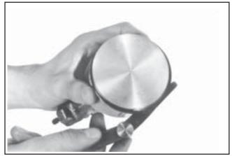
Figure 10-10. Measuring Piston Ring Side Clearance.
