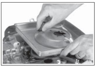
Figure 9-10. Removing Breather Tube from Base.
