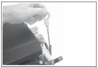
Figure 9-2. Removing Dipstick from Tube.
