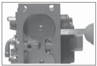
Figure 5-31. Checking Float Height.
