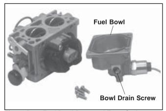
Figure 5-16. Fuel Bowl Removed From Carburetor.
