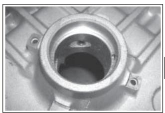
Figure 11-1. Seal Bore of Crankcase.
