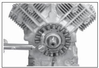
Figure 11-23. Torquing Stator Screws.
