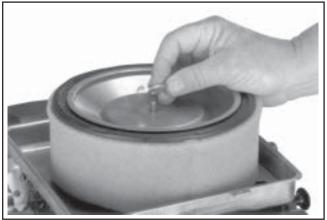
Figure 4-5. Removing Element Cover Wing Nut.
