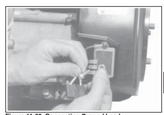
Figure 11-69. Connecting Ground Lead.
