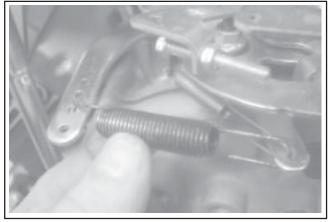
Figure 11-85. Connecting Spring to Governor Lever.
