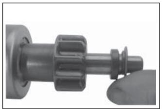
Figure 8-62. Installing Thrust Washer.
