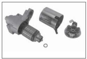
Figure 8-50. Starter Frame Removed.
