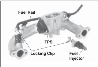
Figure 5B-33. Manifold Assembly.
