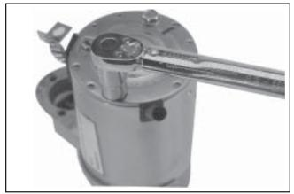
Figure 8-71. Torquing Thru Bolts.
