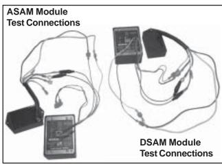
Figure 8-14. Connected Tester Leads.
