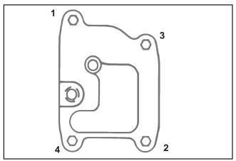
Figure 11-68. Breather Cover Fastener Torque Sequence.
