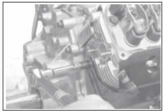
Figure 11-66. Tighten Baffle Mounting Screws.
