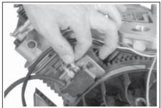
Figure 9-47. Position of SMART-SPARK<sub>™</sub> Ignition Module.
