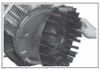
Figure 9-61. Removing Fan.
