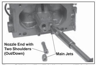
Figure 5-27. Installing Main Nozzles and Main Jets.
