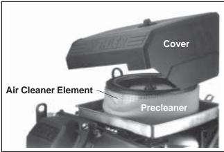
Figure 4-3. Removing Knob Style Cover.
