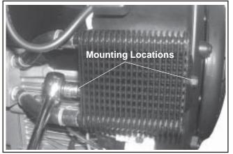
Figure 11-100. Mounting Oil Cooler (Blower Housing Mounted Cooler).
