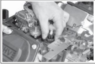
Figure 11-88. Installing Oil Sentry™ Switch.
