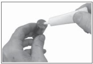
Figure 11-34. Applying Camshaft Lubricant to Bottom of Lifters.
