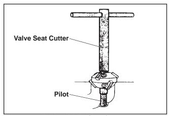
Figure 10-7. Typical Valve Seat Cutter.
