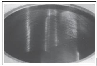
Figure 10-3. Cylinder Bore Crosshatch after Honing.
