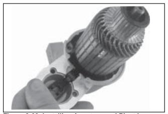
Figure 8-63. Installing Armature and Pivot Lever.
