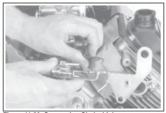
Figure 11-83. Connecting Choke Linkage.
