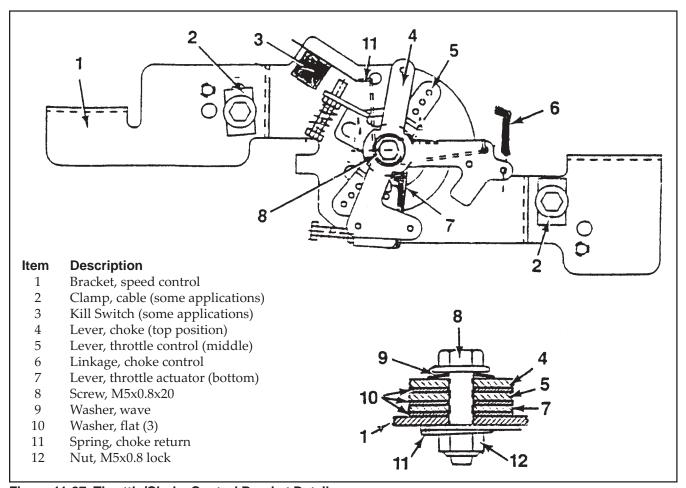
Figure 11-87. Throttle/Choke Control Bracket Detail.
