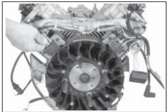
Figure 9-46. Disconnecting Leads from Ignition Modules.
