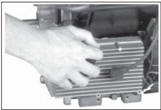
Figure 11-102. Hand Tightening Oil Filter.
