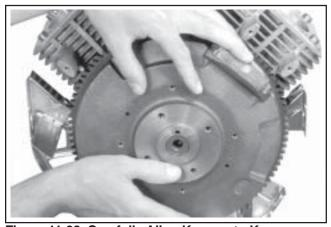
Figure 11-28. Carefully Align Keyway to Key.
