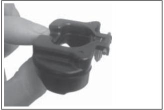
Figure 5-18. Float and Inlet Needle Details.
