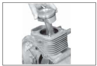
Figure 9-72. Removing Piston/Connecting Rod Assemblies.
