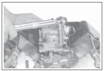
Figure 11-76. Installing Carburetor Assembly.
