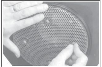
Figure 11-67. Installing Metal Type Grass Screen.
