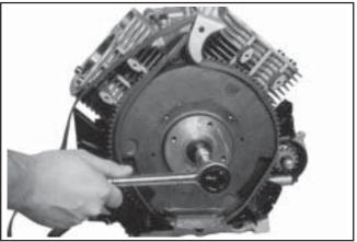
Figure 9-62. Removing Flywheel Fastener Using Strap Wrench.
