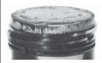
Overheated or Deteriorated Oil
