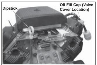
Figure 6-2. Location of Oil Fill Cap and Dipstick.
