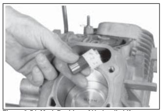
Figure 9-54. Mark Position of Hydraulic Lifters.
