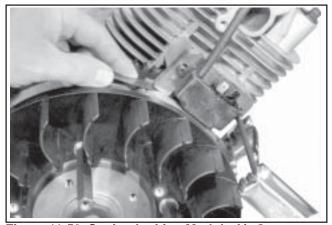
Figure 11-50. Setting Ignition Module Air Gap.
