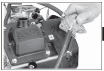
Figure 9-19. Remove Fuel Pump and Lines.
