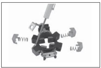
Figure 8-68. Removing Retaining Clips.
