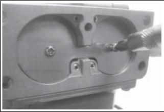
Figure 5-37. Installing Choke Plate.
