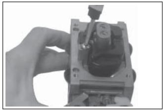
Figure 5-30. Installing Float Assembly.
