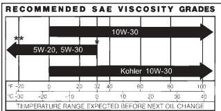
\*Use of synthetic oil having 5W-20 or 5W-30 rating is acceptable, up to  $4^{\circ}$ C ( $40^{\circ}$ F).
