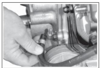
Figure 9-16. Disconnecting Pulse Line from Crankcase.
