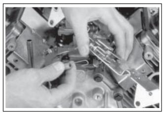
Figure 9-23. Disconnecting Spring from Bracket.
