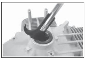
Figure 9-77. Removing Oil Seal.
