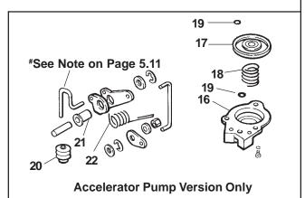
Figure 5-11. CH18-740 Carburetor – Exploded View.
