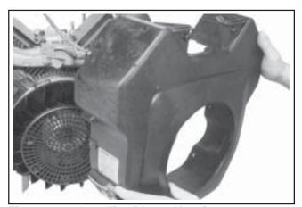
Figure 11-61. Installing Blower Housing.
