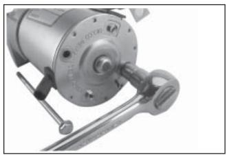
Figure 8-48. Removing Thru Bolts.
