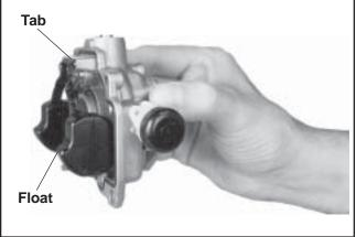
Figure 5-10. Carburetor Float Adjustment.
