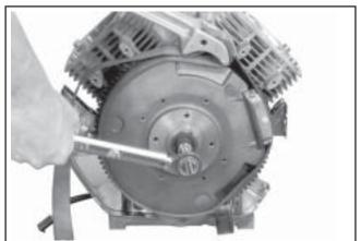
Figure 11-29. Installing and Torquing Flywheel Fastener.
