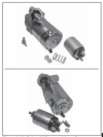
Figure 8-46. Solenoid Removed from Starter.
