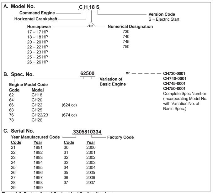
Figure 1-2. Explanation of Engine Identification Numbers.
