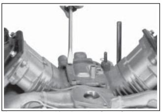
Figure 9-41. Breaking Breather Cover Seal.
