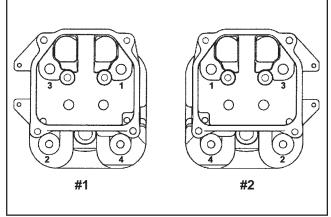
Figure 11-42. Cylinder Head Fastener Torque Sequence.
