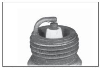
**Overheated:** Chalky, white deposits indicate very high combustion temperatures. This condition is usually accompanied by excessive gap erosion. Lean carburetor settings, an intake air leak, or incorrect spark timing are normal causes for high combustion temperatures.
