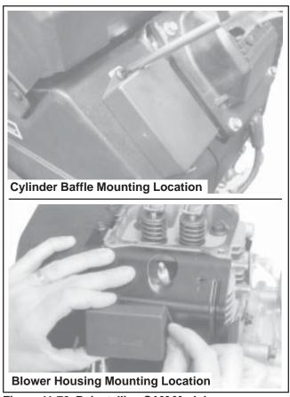
Figure 11-72. Reinstalling SAM Module.
