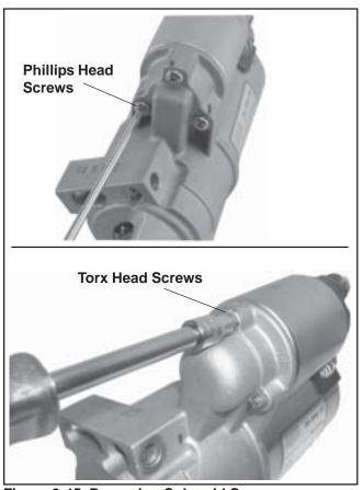
Figure 8-45. Removing Solenoid Screws.
