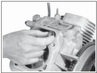
Figure 11-35. Installing Hydraulic Lifters.
