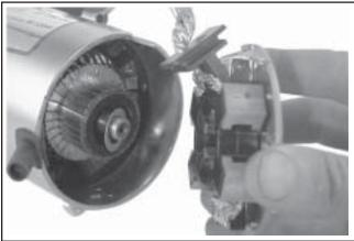
Figure 8-49. Removing Commutator End Plate Assembly.
