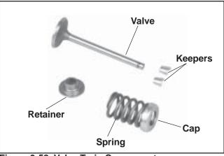
Figure 9-58. Valve Train Components.
