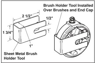
Figure 8-40. Brush Holder Tool (Style "A" End Cap).
