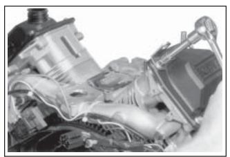
Figure 9-45. Removing Valve Covers.
