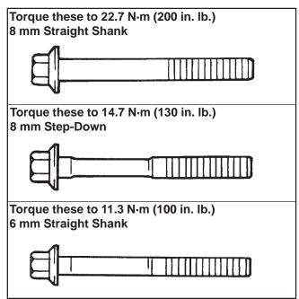
Figure 11-10. Connecting Rod Bolts.
