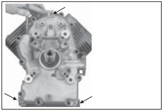
Figure 9-67. Location of Three Splitting Tabs.
