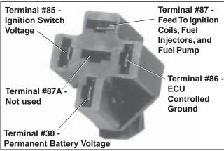
Figure 5B-14. Relay Connector.
