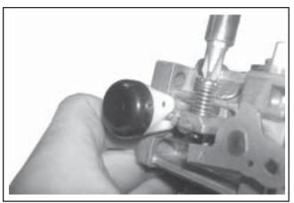
Figure 5-28. Installing Idle Speed Adjusting Screw and Spring.
