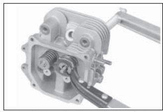
Figure 9-57. Removing Valves with Valve Spring Compressor.
