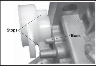
Figure 5-34. Assembling Choke Lever.
