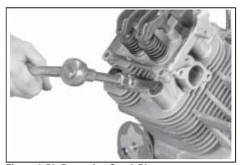
Figure 9-50. Removing Spark Plugs.
