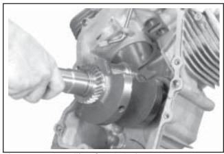
Figure 11-7. Installing Crankshaft.
