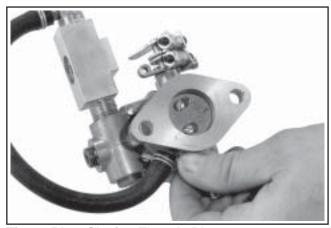
Figure 5A-9. Closing Throttle Plate.
