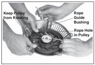
Figure 7-3. Installing Rope.
