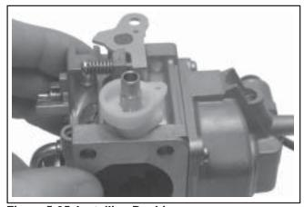
Figure 5-35. Installing Bushing.
