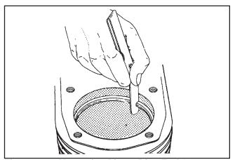
Figure 10-9. Measuring Piston Ring End Gap.
