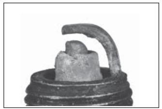
**Worn:** On a worn plug, the center electrode will be rounded and the gap will be greater than the specified gap. Replace a worn spark plug immediately.
