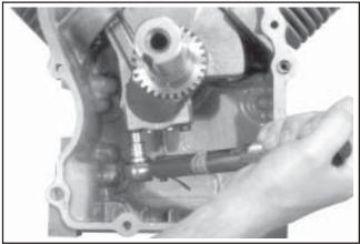
Figure 11-11. Torquing Connecting Rod End Cap.
