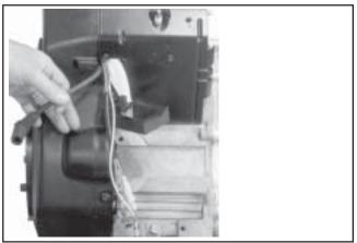
Figure 11-63. Routing Wiring Harness and Leads.
