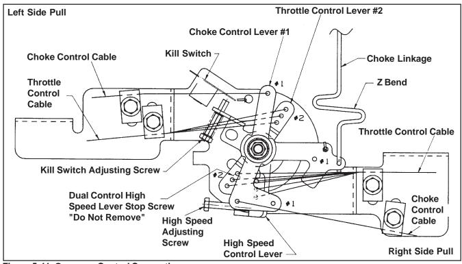
Figure 5-41. Governor Control Connections.
