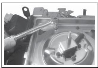
Figure 11-95. Tightening Rear Base/Bracket Screws (Some Models).
