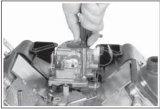
Figure 9-27. Removing Carburetor Mounting Screws.
