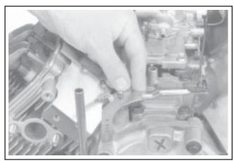
Figure 11-80. Install Governor Lever to Shaft.
