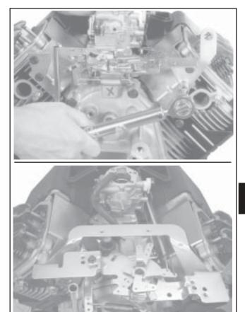
Figure 11-84. Torquing Main Control Bracket.
