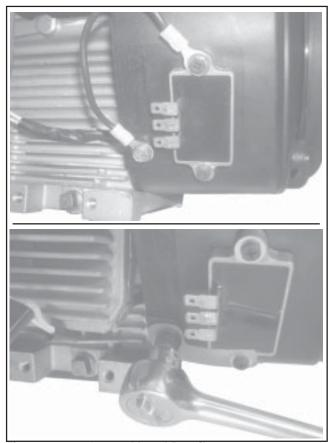
Figure 11-64. Ground Lead Details.
