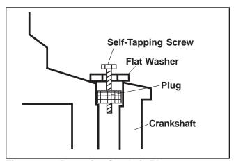
Figure 10-2. Removing Crankpin Plug.
