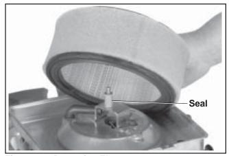
Figure 4-6. Removing Elements.
