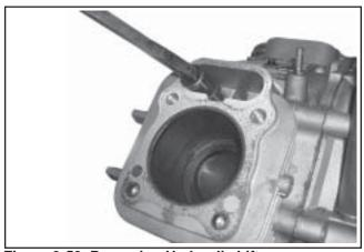
Figure 9-53. Removing Hydraulic Lifter.
