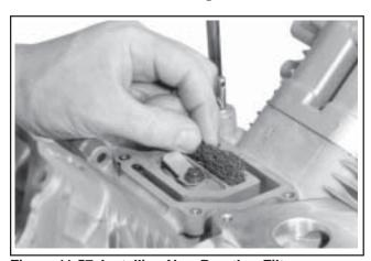
Figure 11-57. Installing New Breather Filter.
