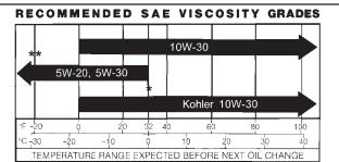
\*Use of synthetic oil having 5W-20 or 5W-30 rating is acceptable, up to 4°C (40°F).
