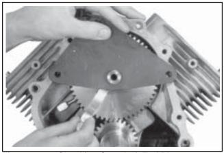
Figure 11-14. Checking Camshaft End Play.
