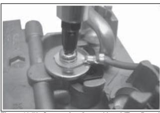
Figure 11-79. Connecting Ground Lead (Two-Barrel Carburetor).
