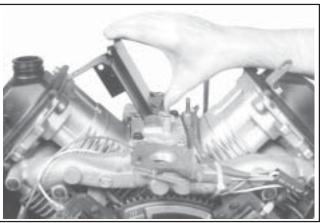
Figure 9-40. Removing Inner Baffles.
