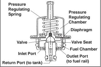
Figure 5B-29. Fuel Pressure Regulator Details.
