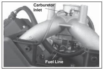
Figure 11-96. Breather Hose and Fuel Line Details.
