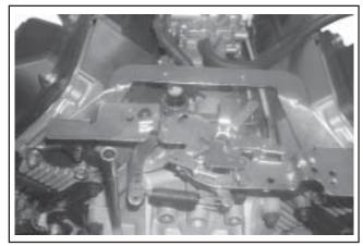
Figure 9-22. Rear Air Cleaner Bracket (Some Models).
