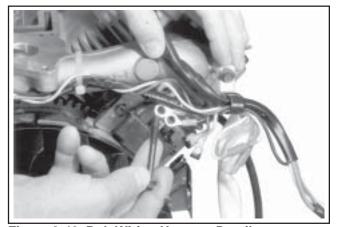
Figure 9-49. Bolt Wiring Harness Detail.
