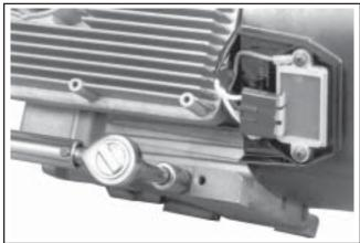
Figure 11-103. Reinstall and Torque Both Oil Drain Plugs.
