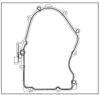
Figure 11-19. Closure Plate Sealant Pattern.
