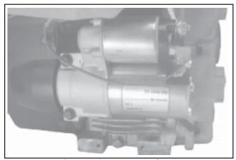
Figure 11-74. Connecting Leads to Starting Motor.
