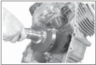
Figure 9-73. Removing Crankshaft.
