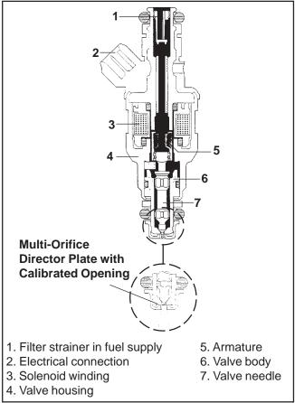
Figure 5B-18. Fuel Injector Details.
