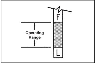
Figure 6-3. Oil Level Marks on Dipstick.
