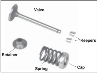
Figure 11-38. Valve Components.
