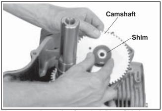
Figure 9-69. Removing Camshaft (Note Shim).
