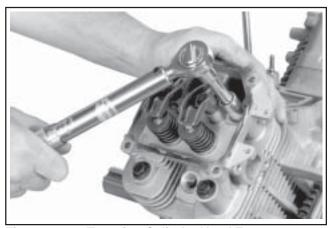
Figure 11-41. Torquing Cylinder Head Fasteners.
