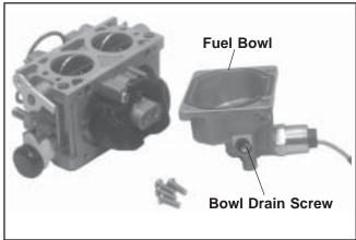
Figure 5-22. Fuel Bowl Removed From Carburetor.
