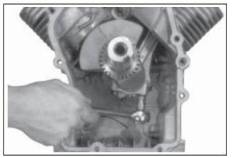
Figure 9-70. Removing Connecting Rod Bolts.
