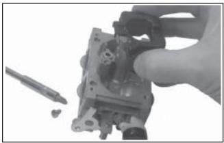
Figure 5-23. Removing Float and Inlet Needle.
