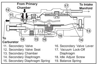
Figure 5A-22. Secondary Chamber.
