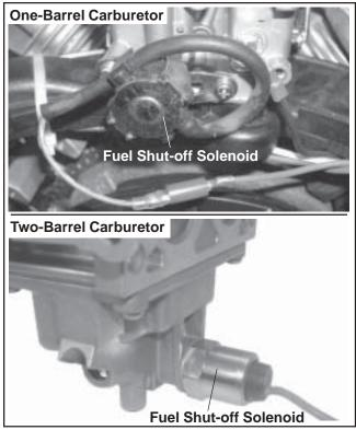
Figure 5-4. Fuel Shut-off Solenoid.
