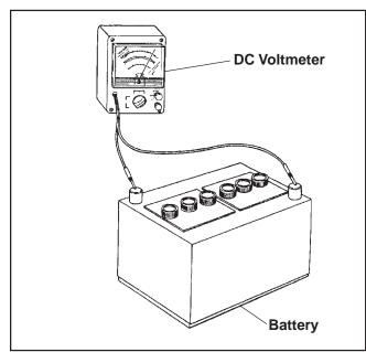
Figure 8-2. Battery Voltage Test.
