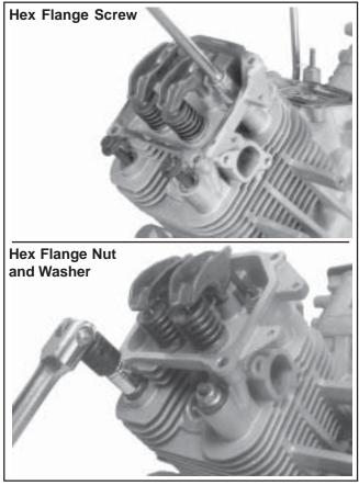
Figure 9-51. Removing Cylinder Head Fasteners.
