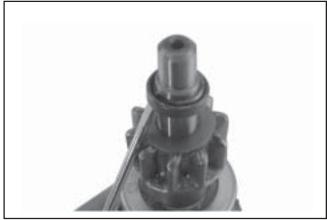
Figure 8-61. Installing Stop Collar and Retainer.
