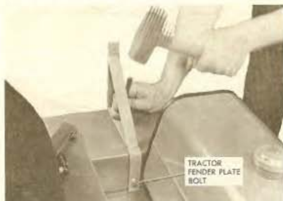
FIG. 5 Install Rear Mounting Brackets
