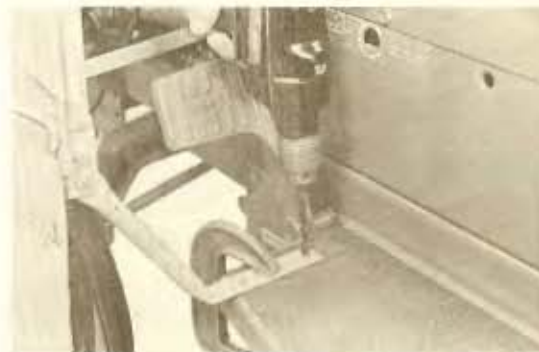
FIG. 10. Secure Foot to Footrest
