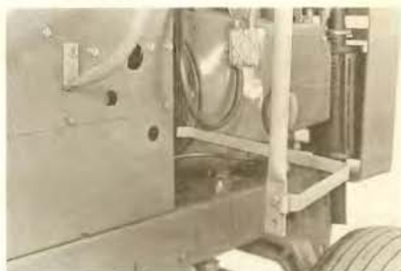
FIG. 3 Attach Right Foot Pocket Guard and Door Hinge
