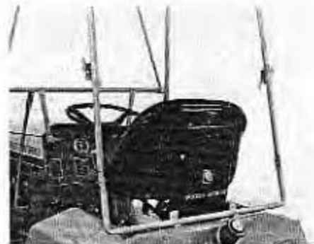
FIG. 10. Install Rear Corner Posts
